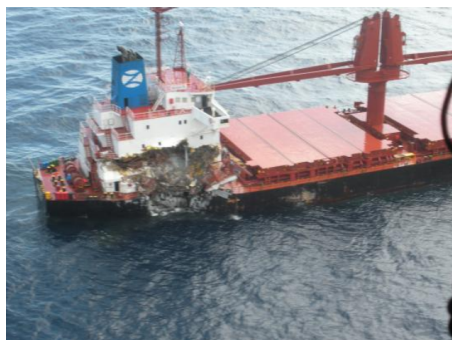
Figure 6.2: A vessel after a collision, from (The Maritime Executive, 2012a)
