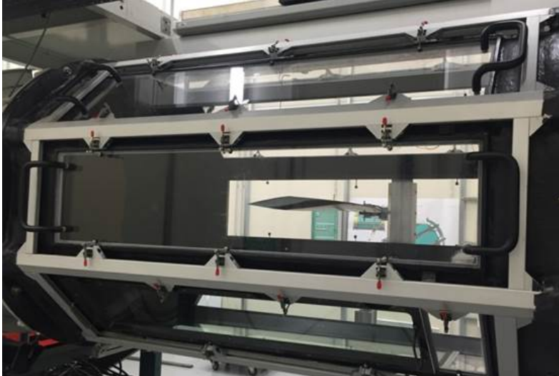
Figure 2.1. Wall-mounted blade in the S2L optical test section.
