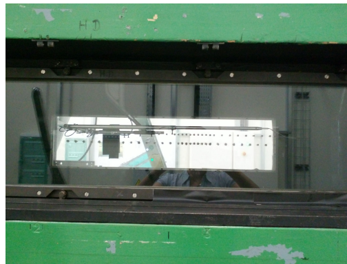
Figure 3.2. Prandtl antenna mounted on the travel system in the wooden test section.
