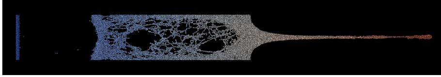
Figure 6.4 | Ejection of matter at the reflection of the shock on the free surface.
