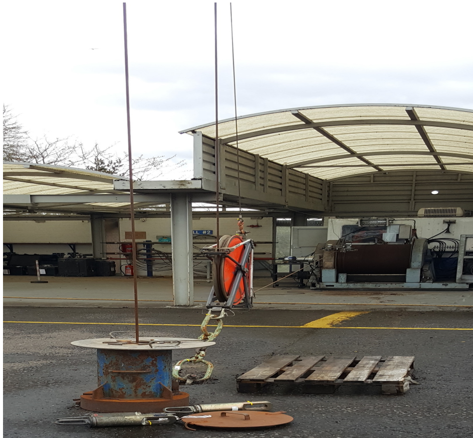
Figure 4.8: The set-up of the field test in Livingston. The DAS cable is lowered down the borehole from a winch visible in the background of the image.
