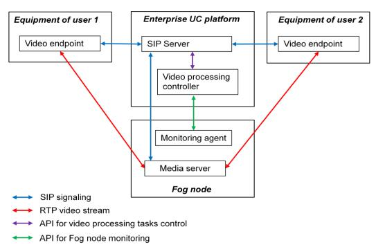
Figure 4.1: Structure of DGC standalone system
