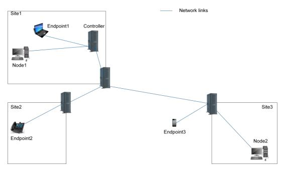
Figure 4.2: Topology for example of ALTO usage
