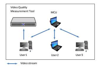
Figure 6.1: Configuration of the testbed: User1 receives video stream from the MCU and via HDMI connection sends it to the Video Quality Measurement Tool
