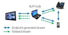
Figure 2.14: Conference topology based on Application Level Multicast
