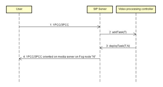
Figure B.1: Task "T" is added to the system and Video processing controller selects Fog node "N" for execution. Then SIP Server notifies conference participants that media server is on the node "N" where they should send their video streams.
