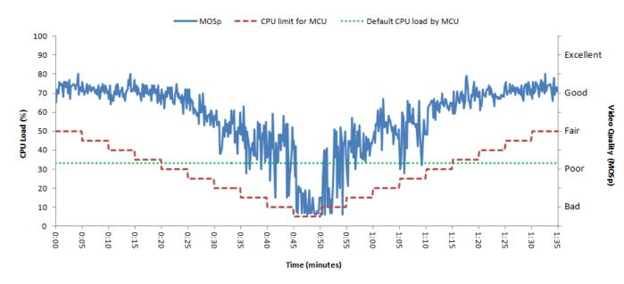
Figure 6.4: Video quality affected by launching 3rd party process competing with MCU process for CPU resources
