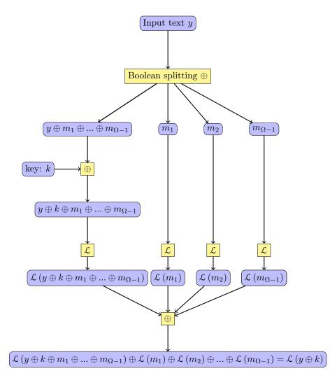
Figure 1.2: Schematic of a linear part of a masking scheme of a block cipher.
