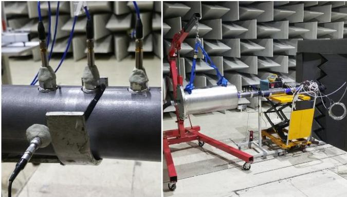
Figure 5: Left: 3 pressure sensors (vertical) and the Microflow sensor (horizontal). Right: global view of the experimental rig.
