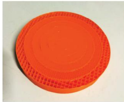
Fig. 2.27 Dielectric focusing lens in Ku-band realized using extrusion 3D printing [90].
