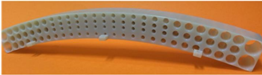
Fig. 2.30 3D printed dielectric superstrate for restoring in phase emission from non-planar microstrip array [95].
