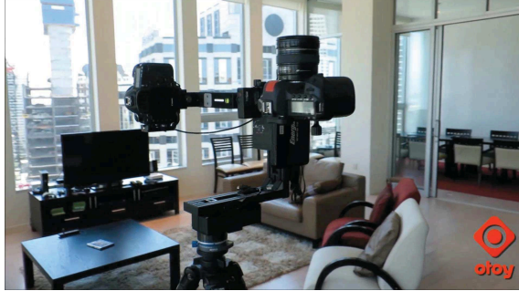
Figure 2.2: Still light-field capture system (Otoy) based on a single moving camera [32].
