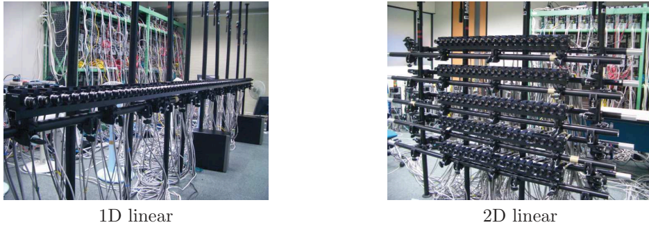
Figure 2.6: Fujii Laboratory camera arrays at Nagoya University [40]
