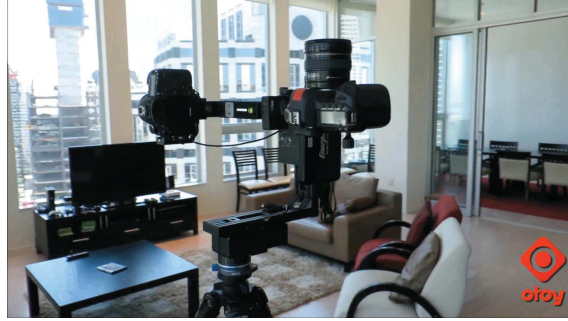
Figure 2.2: Still light-field capture system (Otoy) based on a single moving camera [32].
