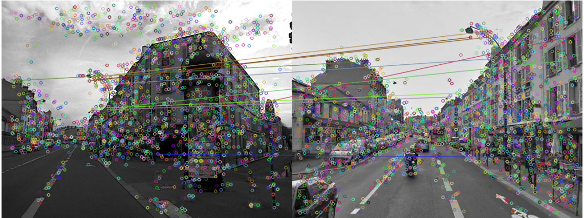
Figure 6.18: Final inliers detected by the SURF-SURF feature in Scenario #2. A lot of matches are detected but there are still false matches.
