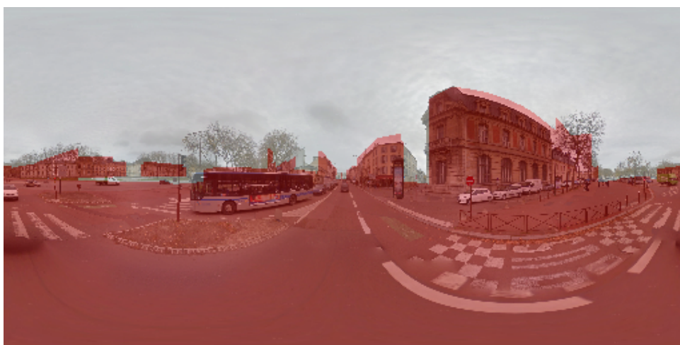
Figure 5.12: Example of the discrepancy between panorama and depth map of Figure 5.5. The red area illustrates the coverage of depth map without value 0.
