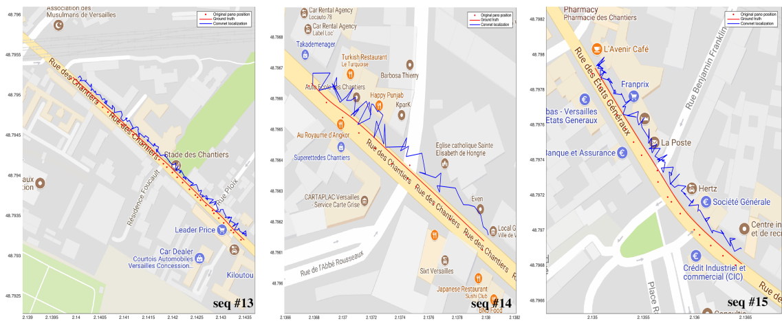
Figure 9.23: The localization output from sequence No. 13, 14 and 15 obtained by the convnet method. The original panorama position, the ground truth and the convnet results are noted in red point, red line and blue line respectively.
