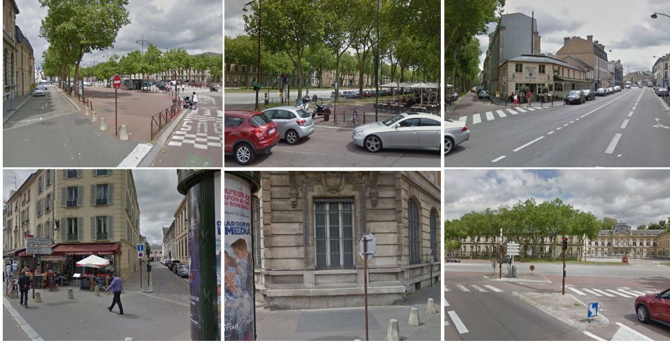
Figure 5.15: Rectilinear images are back projected from the panorama in Figure 5.11 with local yaw angle \eta changing by [0^\circ, 60^\circ, \dots, 360^\circ] . The virtual cameras' FoV, focal length and resolution are all the same as the online camera MIPSEE.
