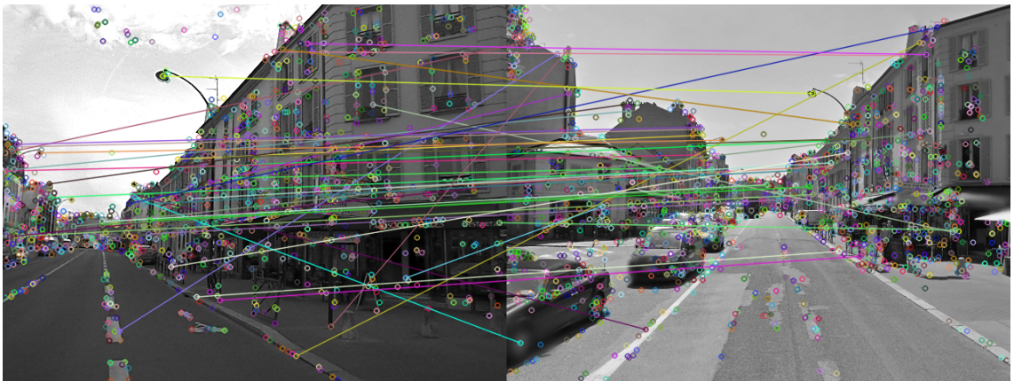
Figure 6.7: FLANN matching with SIFT-SIFT features after the ratio test and symmetric check.
