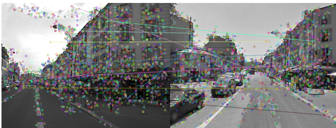
Figure 6.17: Final inliers detected by the SURF-SURF feature in Scenario #1. SURF feature works in normal point view but some wrong matches exist due to the repetitive elements in the urban environment.
