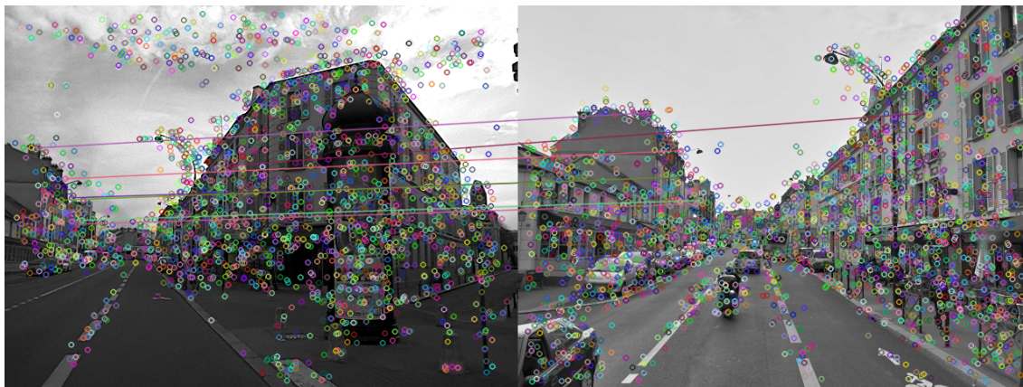
Figure 6.15: Final inliers detected by the SURF-SIFT feature in Scenario #2. SURF-SIFT still performs well for big different viewpoint but the detected number is small.
