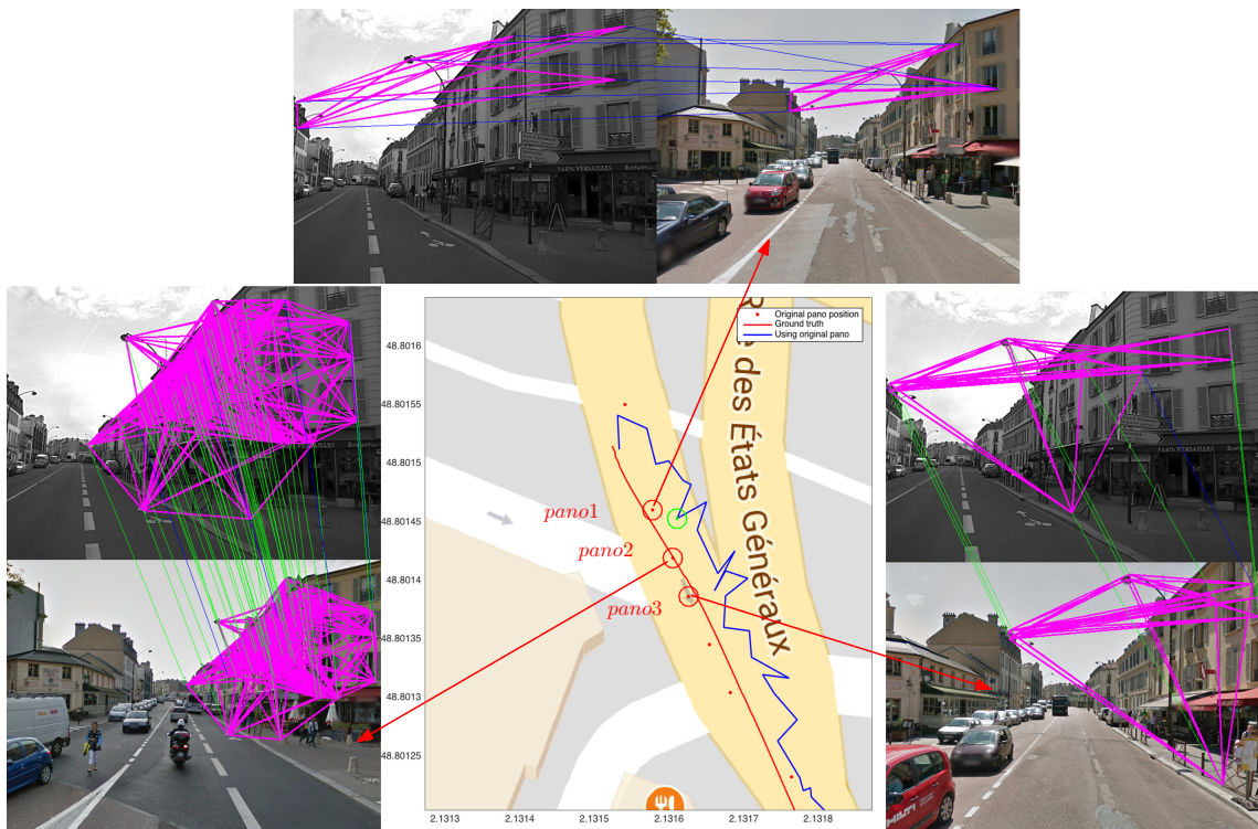
Figure 7.11: An example of 2 pairs of validated matches between a monocular image and its retrieved Street View images by kVLAD descriptors. The positions of Street Views and the estimated localization are displayed in red and green circles respectively. kVLAD matches verified by ORSA are the green lines and those verified by graph matching are the blue lines.
