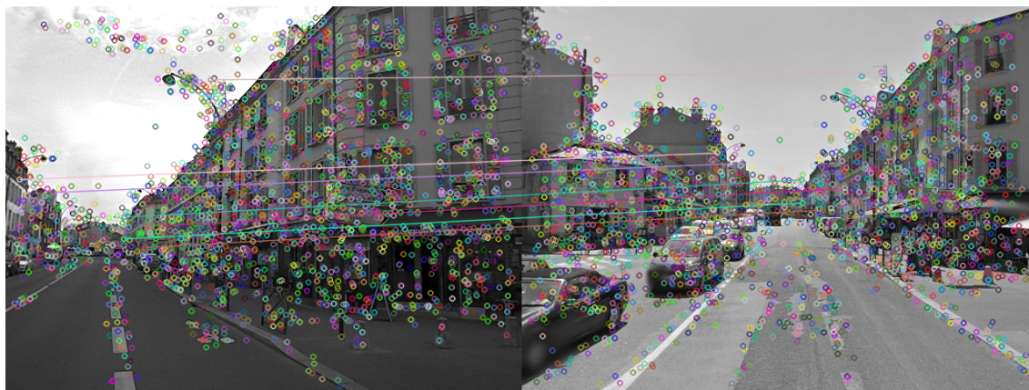
Figure 6.14: Final inliers detected by the SURF-SIFT feature in Scenario #1. As the matches are correct and enough, SURF-SIFT works well in normal point view.
