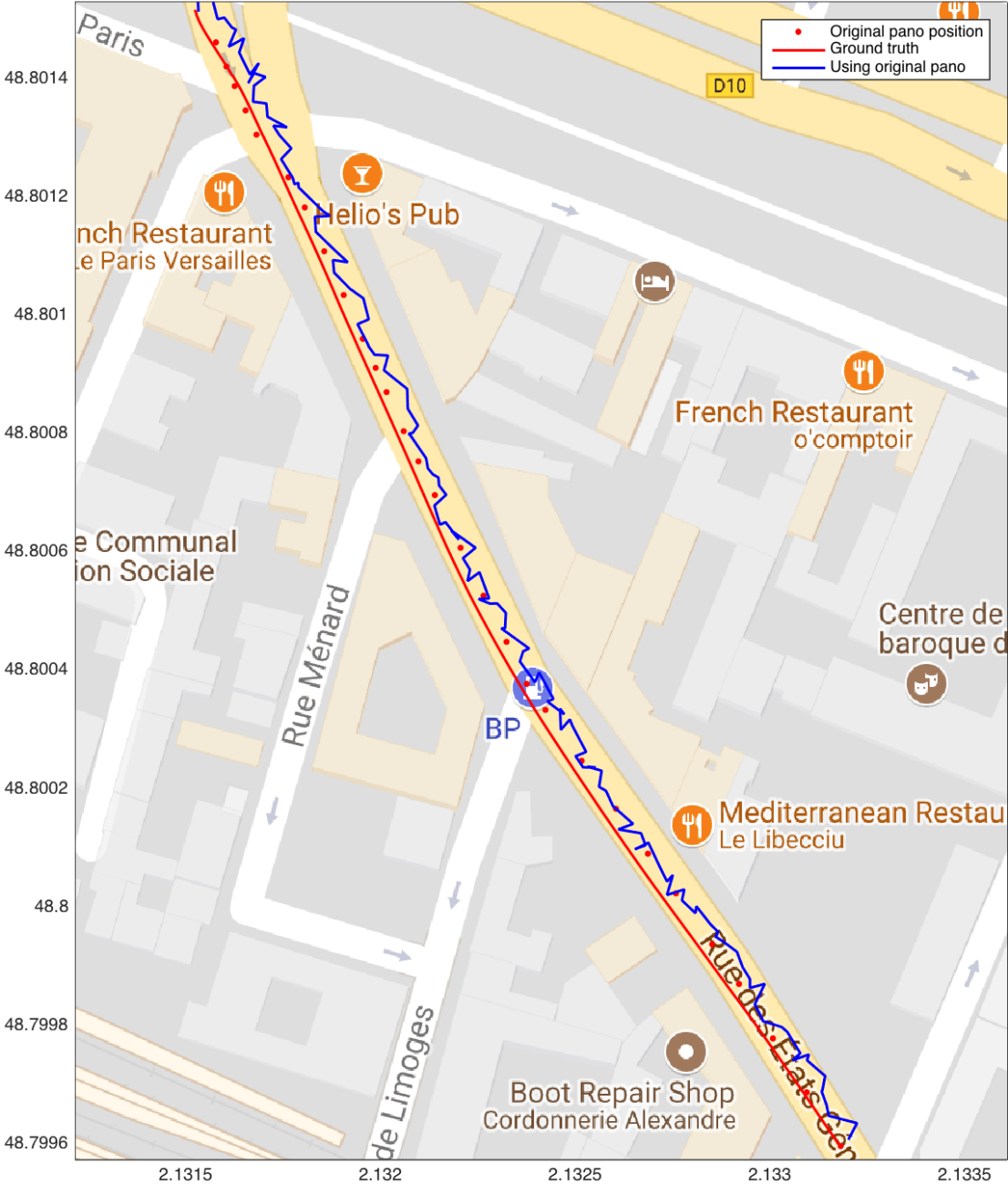
Figure 7.10: Bird’s-eye view of the metric global localization. The red points represent the locations of the Street View cameras. The red and blue lines mark RTK-GPS ground truth and the estimated positions of the monocular camera respectively.
