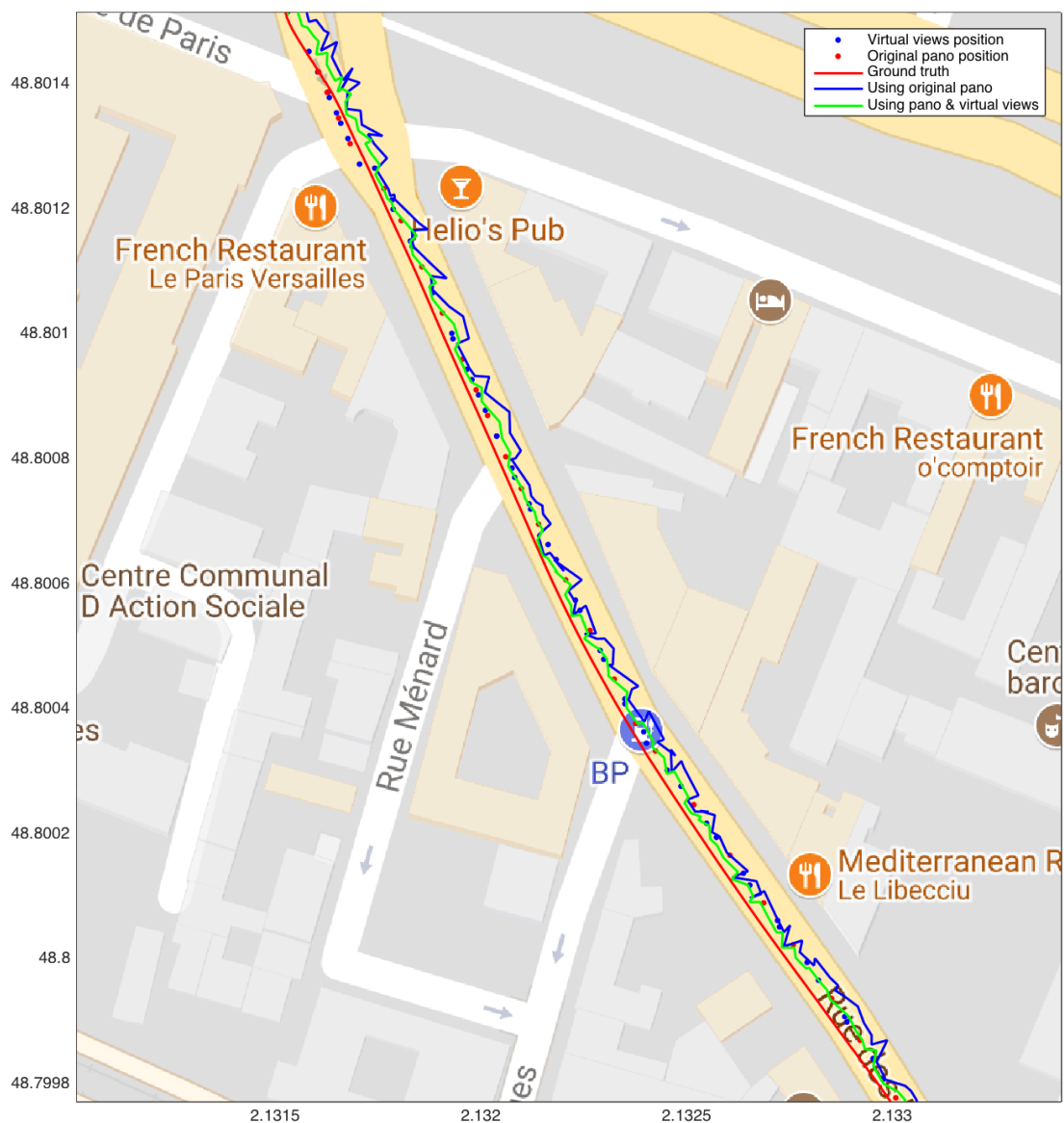
Figure 7.17: The output from a single localization run using original Street Views and synthesizing virtual views: The trajectories obtained with/without virtual views are plotted in green/ blue respectively. The ground truth in red line is recorded by a centimeter-level RTK GPS.
