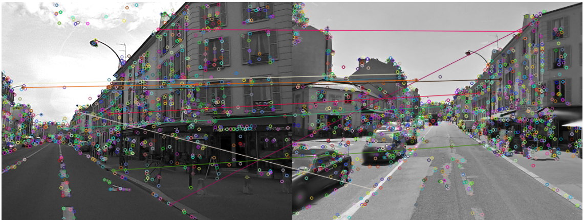
Figure 6.8: FLANN matching with SIFT features after ratio test, symmetric check and 8-point RANSAC selection.
