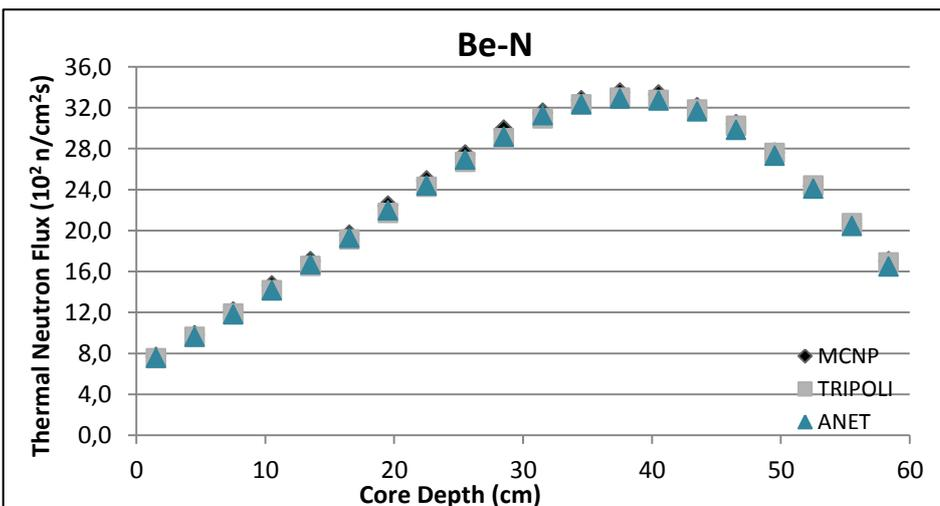
**Figure 6.8a:** Thermal neutron flux profile in reflector Be-N by ANET vs two independent stochastic results.
