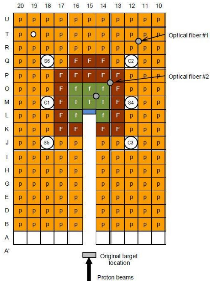
**Figure 5.11b:** Core configuration case V of KUCA.
