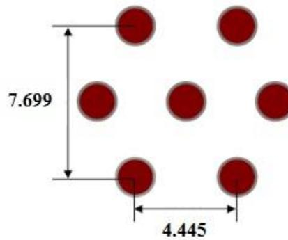
**Figure 5.4:** The unit of the TNR-AUTH hexagonal lattice (dimensions in cm).
