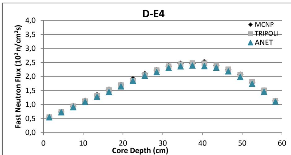
**Figure 6.7c:** Fast neutron flux profile in dummy assembly D-E4 by ANET vs two independent stochastic results.
