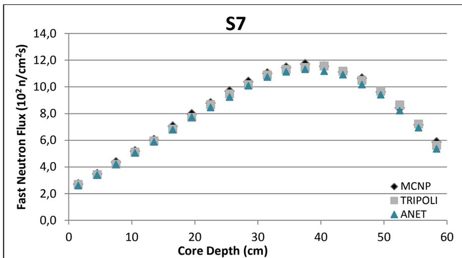
**Figure 6.6c:** Fast neutron flux profile in fuel assembly F-S7 by ANET vs two independent stochastic results.
