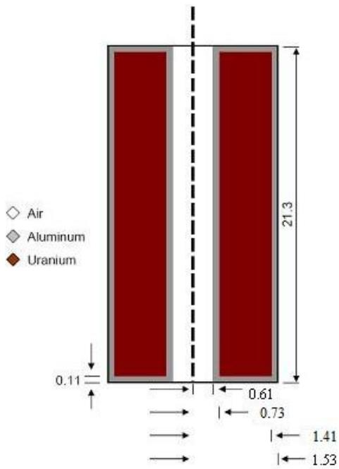
**Figure 5.3:** Description of the TNR-AUTH fuel slug (dimensions in cm).
