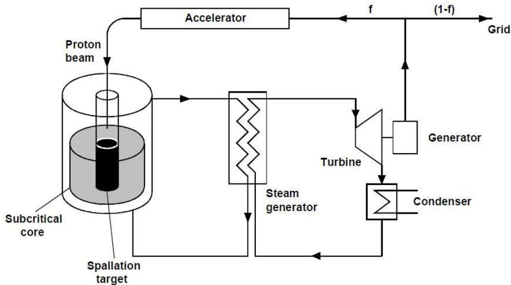
**Figure II.1:** Concept of an accelerator-driven system.
