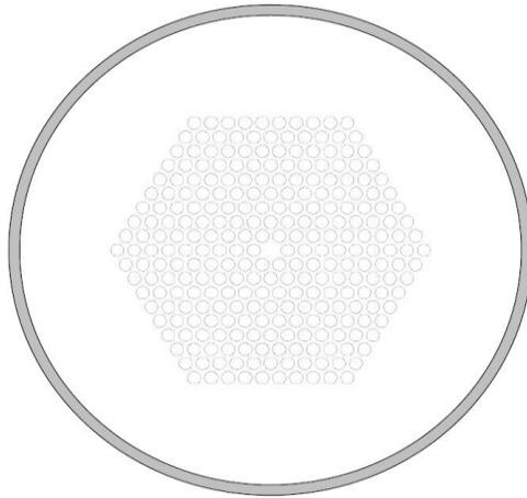
**Figure 5.5:** Full hexagonal lattice arrangement of the TNR-AUTH.
