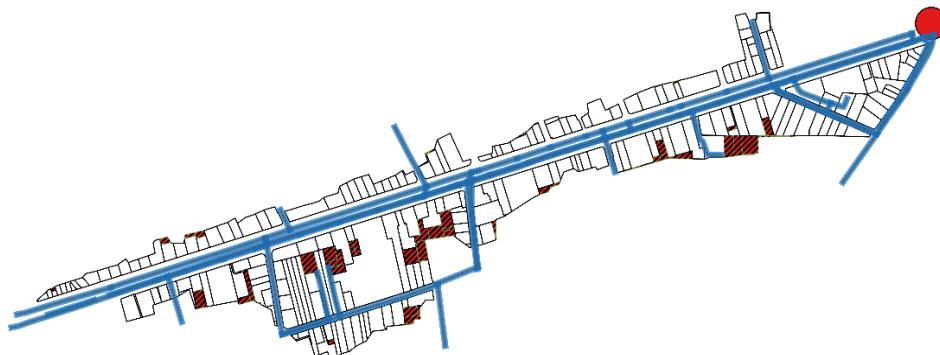
Fig. 3 Cadastral parcels of "Le Perreux" catchment. White parcels represents the UHEs including a fraction of the adjacent street. Red dashed parcels represent isolated UHEs. The blue lines and the red circle represent respectively the segments of the hydrological network and the catchment outlet.
