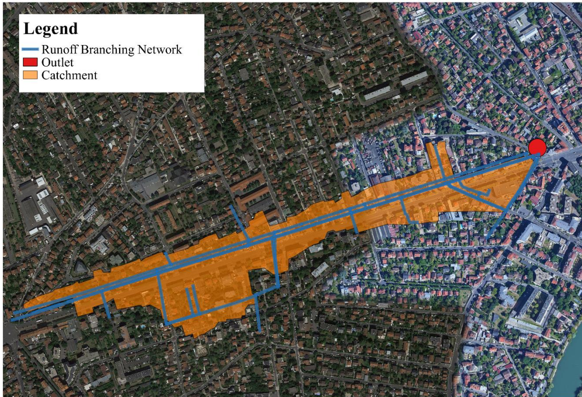
Fig. 2 The studied catchment and the runoff branching network (including both street and sewer segments). The red point represents the outlet of the catchment.
