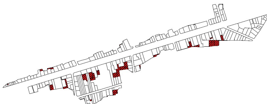
Fig. S2 The spatial discretization of the basin in terms of UHE. The white parcels represents the UHEs including a fraction of the adjacent street. Red dashed parcels represent internal UHE.
