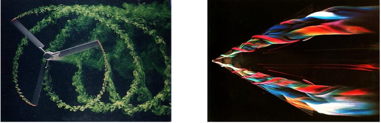
Figure 1.3: Hydrodynamic tunnel visualization of a helicopter rotor wake (left) and the leading edge vortices formed due to the flow separation at the apex of a thin delta wing (right). H. Werlé, ONERA [60, 225].
