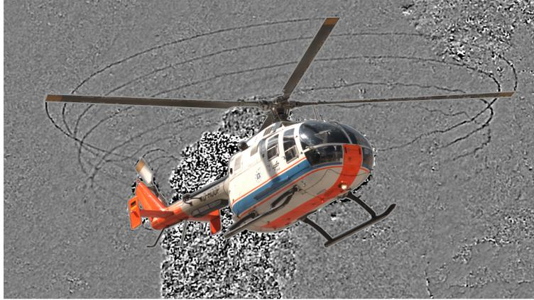
Figure 1.1: Photograph of a BO105 light utility helicopter during a swinging maneuver and visualization of the blade-tip vortices by a background-oriented schlieren (BOS) technique. A. Bauknecht et al. [12].
