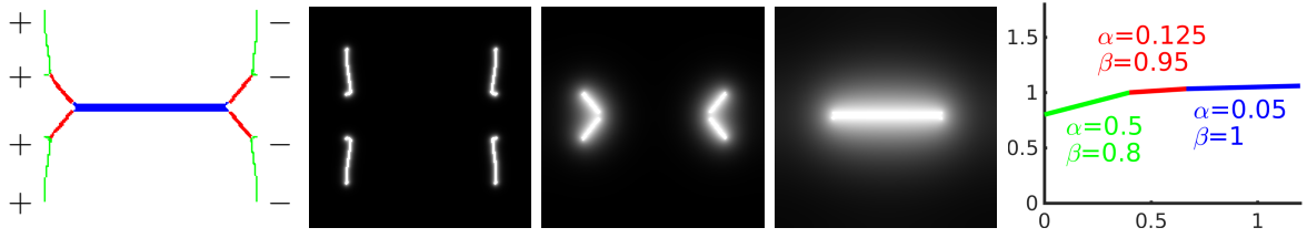
Figure D.6: Computed mass flux \sigma and phase fields \varphi_1, \varphi_2, \varphi_3 for the cost function shown on the right, \varepsilon = 0.005 . The color in \sigma indicates which phase field is active. The result is obtained by optimizing the functional defined in Chapter Three .
