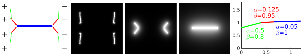
Figure 6: Computed mass flux \sigma and phase fields \varphi_1, \varphi_2, \varphi_3 for the cost function shown on the right, \varepsilon = 0.005 . The color in \sigma indicates which phase field is active. The result is obtained by optimizing the functional defined in Chapter Three .
