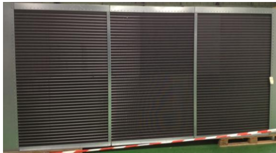
Fig. 4: Fin-and-tube heat exchanger mounted at Source “A”
