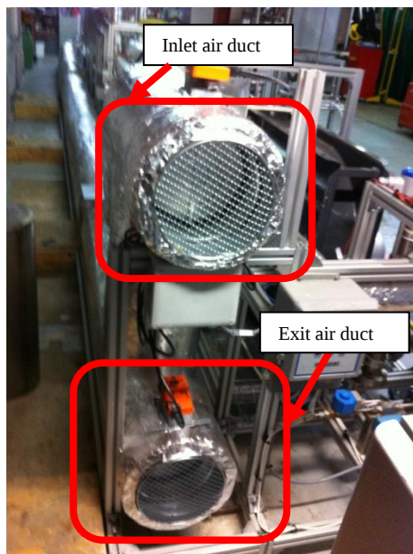
Fig. E.9: Inlet, exit, and re-circulated air ducts
