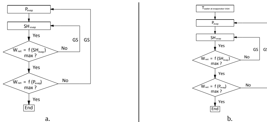
Fig. C.2: Optimization algorithms for simple ORC with : (a) indirect-contact condensation (direct evaporator), (b) both direct and indirect (indirect evaporator)-contact condensation
