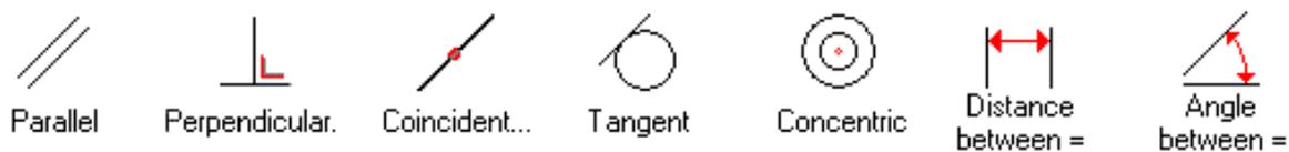
Figure 1.9: Example of some geometric constraints
