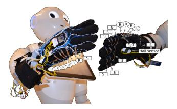
FIGURE 5.1: Sensor positions on the Pepper's glove. Note: The S and R annotations correspond to the role attributions given in Appendix A for the humans gloves.
