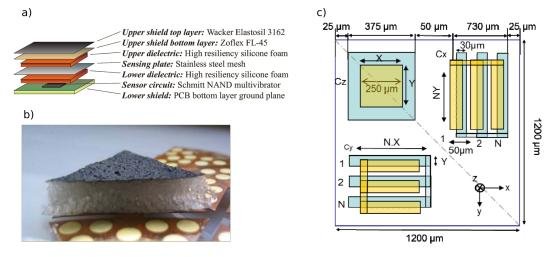
FIGURE 2.6: a) Schematic of a piezo-capacitive cell (extracted from Ulmen and Cutkosky, 2010); b) Picture of a module with 12 piezocapacitive cells (extracted from Cannata et al., 2008); c) Schematic of a 3D piezo-capacitive cell, composed with 3 sub-cells (extracted from Nazeer, 2012)
