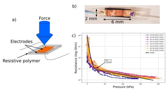
FIGURE 4.9: Design of the piezo-resistive sensors. a) Operating principle, b) picture , and c) calibration laws with corresponding model for one sensor.
