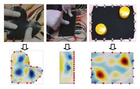
FIGURE 2.9: Examples of Electrical Impedance Tomography (EIT) sensors (extracted from Alirezaei, Nagakubo, and Kuniyoshi, 2007).
