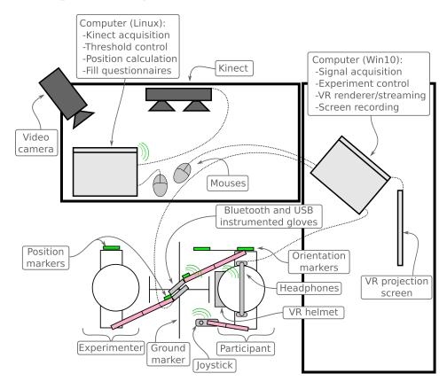
FIGURE 4.11: Global experimental setup
