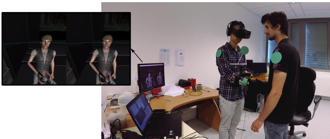
FIGURE 4.12: Example of handshake interaction with the virtual agent, and view of the participant
