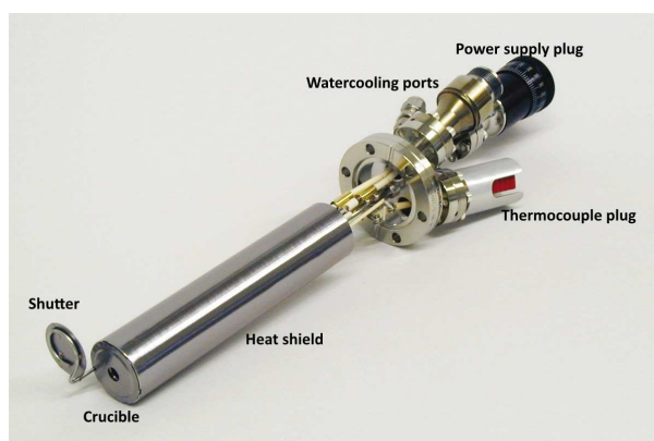
Figure 2.11: Picture of a Knudsen-cell evaporator similar to the one used during my PhD.
