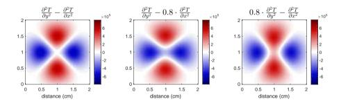
Figure 6.3: The resulting patterns arising when taking the difference between  $\frac{\partial^2 T}{\partial x^2}$ and  $\frac{\partial^2 T}{\partial y^2}$ . Three cases are shown, relatively when  $|\gamma_1| = |\gamma_2|$ ,  $|\gamma_1| < |\gamma_2|$  and  $|\gamma_1| > |\gamma_2|$ .
