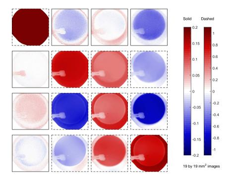
Figure 3.3: The second obtained Mueller matrix  $M_2$ , measured with an applied potential difference (over the 0.5 mm thick BSO) of 1000 volt between the ITO coated circular regions. This makes them distinctively different and observable from the uncoated BSO regions. Same remarks as given in figure 3.2 are valid.
