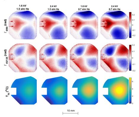
Figure 7.6: The background linear retardances  $\Gamma_{0/90}$  and  $\Gamma_{45/135}$  for the dry air environment in the cases of 700 and 1500 sccm helium flow and an AC voltage amplitude of 1.6 and 2.4 kV. The corresponding (axial) electric field patterns are shown in figure 4.10. The measurements are ordered based on the fitted value of temperature.
