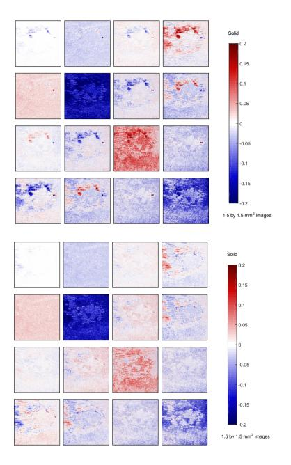
Figure 8.9: The logartihmically decomposed  $L_u$  matrices of the combined sample (BSO + onion cells) under exposure of the AC-driven plasma jet, measured before impact (bottom matrix) and after (top). Depolarization properties are shown in the diagonal elements, while the off-diagnoal elements relate to uncertainties in the optical properties.
