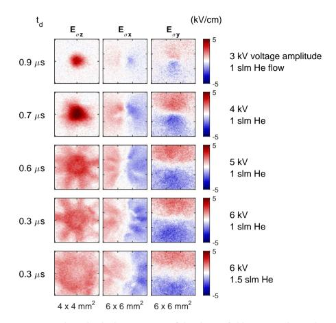
Figure 5.15: The individual components of the electric field patterns obtained at a specific time delay  $t_d$ , relative to the rise of the voltage pulse, while varying the voltage amplitude. Each time delay is part of a time-resolved measurement series, which is shown either in this chapter or in appendix A. The plasma jet is in all cases impacting at 90 degrees at 10 mm from the target.
