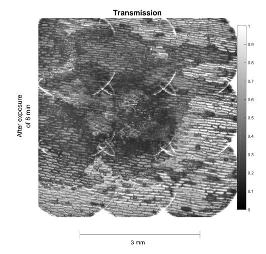
Figure B.4: The mapped transmission relative to air of the combined sample (BSO + onion cells) after 8 minutes of plasma exposure. The ionization waves generated by the plasma jet (2 kV amplitude 30 kHz sine waves and 1 slm helium flow) have impacted in the center of the map, while moving from the right side to the left. This figure is part of figure 8.5, but shown in full scale.
