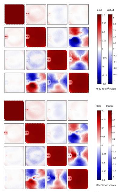
Figure 4.5: The obtained Mueller matrices  $(16 \times 16 \text{ mm}^2 \text{ images})$  of the electrooptic Felinbo examined under normal incidence under exposure of guided ionization waves produced using a plasma jet driven by 30 kHz AC sine waves with 2.0 kV amplitude at 1 slm helium, shown before (top matrix,  $t_d = 1 \ \mu s$ ) and after (bottom matrix,  $t_d = 8.0 \ \mu s$ ) impact of the ionization waves. The colorscale is indicated by the border of the images.
