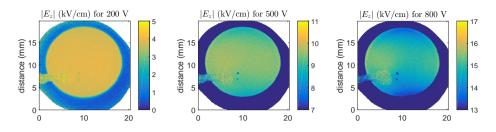
Figure 3.9: The obtained electric field for different applied voltages (sample thickness = 0.5 mm). The color scale is adapted to visualize the possible appearance of the inhomogeneous pattern, which becomes more significant with higher applied voltages.
