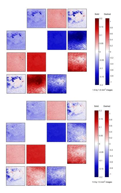
Figure 8.8: The logartihmically decomposed  $L_m$  matrices of the combined sample (BSO + onion cells) under exposure of the AC-driven plasma jet, obtained before impact (bottom matrix) and after (top), showing the diattenuation and birefringent properties. Similar remarks as in figure 8.6 are applicable.
