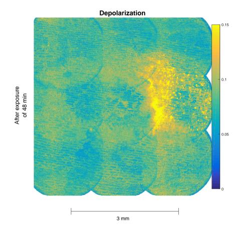
Figure B.11: The mapped total depolarization of the combined sample (BSO + onion cells) after 48 minutes of plasma exposure. This figure is part of figure 8.5, but shown in full scale.
