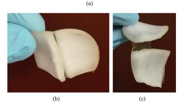
Figure 8.1: An example of the extraction of the single epidermis cell (outer-facing) layer of an onion. The cells offer a cheap and simple test case for the use of Mueller polarimetry to examine more complex plasma surface interactions.
