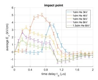
Figure 5.16: The axial electric field averaged in the center of the impact point as a function of time during the high voltage pulse ( $0 \le t_d \le 1.0 \ \mu s$ ) and after ( $t_d > 1.0 \ \mu s$ ) for different voltage amplitudes. The changes are much slower than the increase / decrease of the constant high voltage pulse (50 ns).
