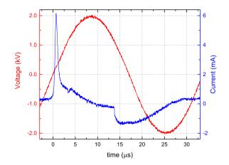
Figure 1.4: The current (blue) measured at the grounded ring electrode when applying the voltage (2 kV sine waves with 30 kHz frequency) to generate the plasma jet. A significant increase of current is obsterved, indicating the ignition around the electrodes, followed by a small *dip* (at 3  $\mu$ s) indicating the moment when the ionization waves propagates in the *plasma plume* area.
