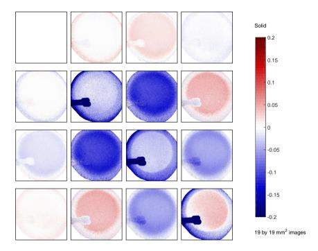
Figure 3.6: The separated depolarization part  $L_{u,1}$  of the logarithmically decomposed matrix L, using measured Mueller matrix  $M_1$ . No voltage difference is applied and similar remarks hold as with the previous figures. Depolarization properties are shown by the diagonal elements, while the off-diagonal elements relate to the uncertainty of the diattenuation and birefringent properties.
