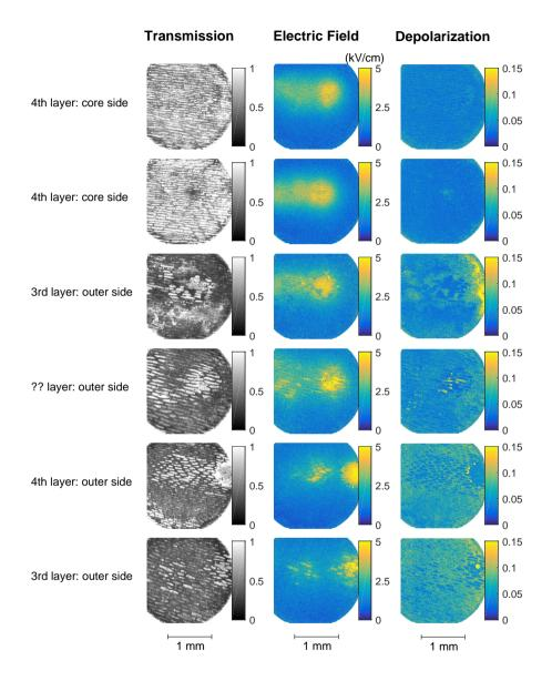
Figure B.1: Repetitive results shown for multiple samples, taking from different onion layers, show comparable results in changes of transmission and depolarization caused by the long-term impact of the ionization waves, which is indicated by the simultaneously obtained electric field pattern. More results are shown in figure B.2.
