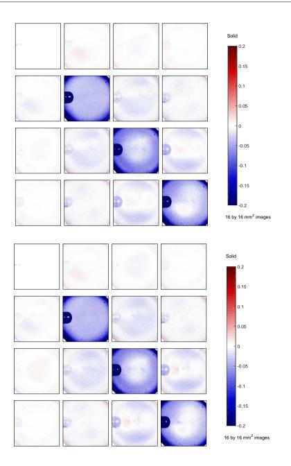
Figure 4.7: Logarithmically decomposed matrices  $L_u$  of the electro-optic Felinbo under exposure of the AC-driven plasma jet, shown before (top) and after impact (bottom). The diagonal elements represent the depolarization properties, while the off-diagonal elements relate to the uncertainty of the diattenuation and birefringent properties.
