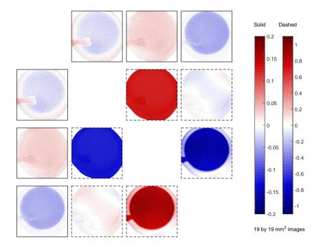
Figure 3.5: The obtained  $L_{m,2}$  matrix using Mueller matrix  $M_2$ , hence including the effect of the applied 1 kV potential difference between the ITO coated regions. Similar remarks hold as discussed in previous figures.
