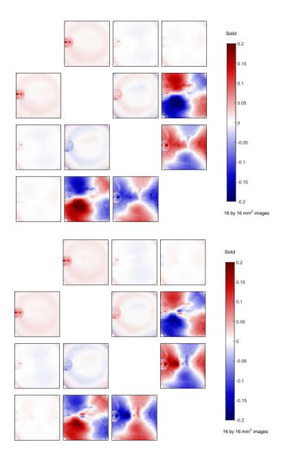
Figure 4.6: Logarithmically decomposed matrices  $L_m$  of the electro-optic Felinbo under exposure of the AC-driven plasma jet, shown before (top) and after (bottom) impact of the ionization waves. Same remarks hold as with the previous figures of  $L_m$ , which only includes the diattenuation and birefringent properties.
