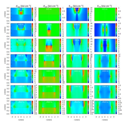
Figure 5.12: The individual electric field contributions caused by  $\sigma$  and  $\rho$  in axial and radial direction as the (numerical) ionization wave approaches and spread on the dielectric surface located at z = 0, calculated by Pedro Viegas using an axysymmetrical numerical fluid model. The pulse ends after 800 ns which causes removal of surface charge in the center of the impact region.
