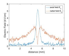
Figure 4.9: The electric field (axial  $E_z$  and radial  $E_y$ ) along a vertical cross-section going through the impact point of the patterns shown in figure 4.8, indicated by the area where  $E_z$  is maximal.
