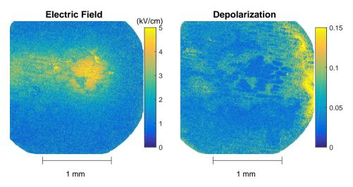
Figure 8.10: The obtained electric field pattern (kV/cm) from the change in linear retardances before and after impact using the logarithmically decomposed time-resolved matrices. The total depolarization is calculated using the second  $L_u$  matrix, relative to the reference measurement of unperturbed BSO without the onion sample present.
