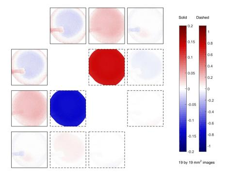
Figure 3.4: The non-depolarizing part  $L_{m,1}$  of the logarithmically decomposed matrix L, using Mueller matrix  $M_1$ . Hence, no voltage difference is applied. The diagonal elements are removed since they do not contain any information due to the separation. The optical properties, diattenuation and birefringence, are included as defined by equation (2.18). Similar remarks hold as discussed in figure 3.2.
