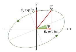
Figure 1.2: Visualization of a polarzation state (red) using an ellipse. This shows the rotating orientation of the oscillations (green) for the electric wave components of the propagating light in the moving plane dependicular to the propagation direction.  $\vec{J_P}$  describes the state of polarization following the Jones calculus.
