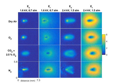
Figure 4.12: The axial and radial electric field patterns (kV/cm) induced inside the electro-optic targets, shown for different operating parameters (columns) of the plasma jet and environmental gas surroundings (rows) in which the ionization waves are travelling towards the targeted material.
