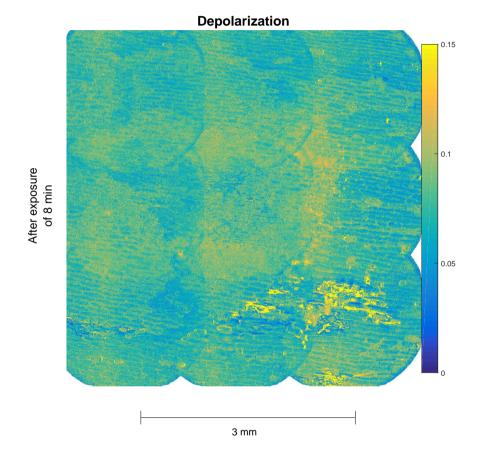
Figure B.10: The mapped total depolarization of the combined sample (BSO + onion cells) after 8 minutes of plasma exposure. This figure is part of figure 8.5, but shown in full scale.
