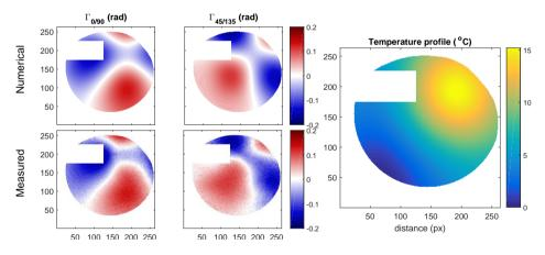
Figure 6.5: The obtained result of the fitting procedure algorithm. After 5000 alterations of a temperature profile have been tested, of which 721 have been accepted as improvement in this example, a temperature profile is obtained shown on the right for which the birefringent outcome matches the measured patterns, shown in the left images. This profile should correspond to the elevation of temperature compared to ambient conditions.
