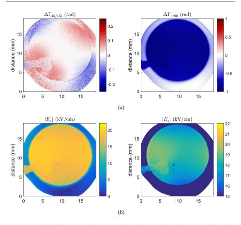
Figure 3.8: The difference in linear retardance due to the application of the voltage potential for both coordinate systems,  $\Delta\Gamma_{0/90}$  and  $\Delta\Gamma_{45/135}$  shown in 3.8(a). These are used to calculate the electric field, using equation (3.29), shown twice with difference color scales in 3.8(b).
