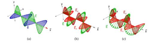
Figure 1.1: The propagation of light in direction  $\vec{k}$  is described by the oscillations of the electric (green) and magnetic (blue) field components in the plane normal to  $\vec{k}$ , see e.g. in figure 1.1(a). For the polarization of the beam the direction and relative phase of the electric field components (red) is considered, referred to as linearly polarized (figure 1.1(b)) or circularly polarized (figure 1.1(c)).
