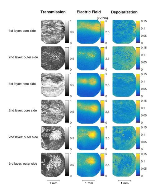
Figure B.2: Similar as figure B.1, here are shown comparable repetitive results, taking from different onion layers, showing changes of transmission and depolarization caused by the long-term impact of the ionization waves, which is indicated by the simultaneously obtained electric field pattern.
