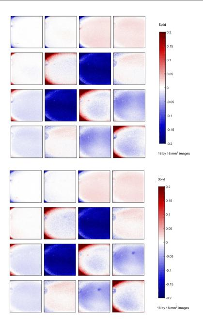
Figure 5.8: Logarithmically decomposed  $L_u$  matrices obtained from the measured Mueller matrices, shown time-resolved for  $t_d = 0.2 \ \mu s$  (top) and  $t_d = 0.7 \ \mu s$  (bottom). The diagonal elements represent the depolarization properties, while the off-diagonal elements relate to the uncertainty of the diattenuation and retardance.
