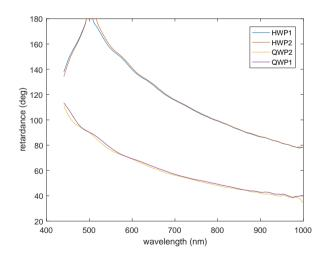
Figure 2.3: The retardance of the liquid crystals obtained spectroscopically using the commerically available *MM16 Spectroscopic Ellipsometer* from *Horiba Jobin Yvon*.
