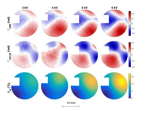
Figure 7.7: The linear birefringent patterns ( $\Gamma_{0/90}$  and  $\Gamma_{45/135}$ ) induced by the pulsed plasma jet operated at different voltage amplitudes. The fitted temperature profiles are shown in the last row. The corresponding time-resolved imaging of light emission and (axial) electric field is shown in chapter 4 section 4.4.3.
