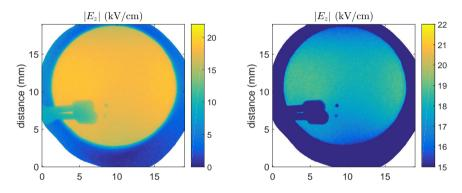
Figure 3.11: The electric field calculated using the linear retardances obtained from the applied homogeneous elliptical retarder model, shown twice with different color scales, which matches the results shown in figure 3.8(b).
