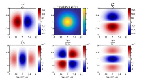
Figure 6.2: The first and second derivatives of a isotropic Gaussian temperature distribution, with an amplitude of 10 °C and standard deviation of 0.5 cm, shown for a  $2 \times 2$  cm<sup>2</sup> area.
