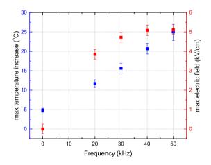
Figure 7.2: Maximum tempeature increase (blue) and maximum (axial) electric field values in the impact piont as a function of operating frequency of the AC driven jet.
