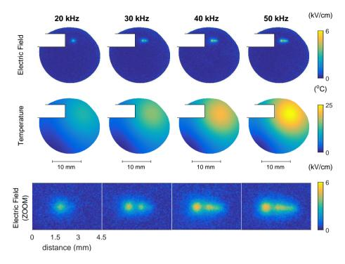
Figure 7.1: The (axial) electric field and temperature pattern induced by the plasma jet in the electro-optic BSO material measured using Mueller polarimetry, for different operating frequencies of the plasma jet. A constant voltage amplitude is used of 2.0 kV, with a helium flow of 1 slm while the horizontally mounted jet is at 7 mm from the target.
