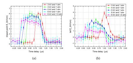
Figure 4.17: Maximum electric field values (kV/cm) observed in the impact point shown in (a) and the field observed in the beginning of the surface *tail* structure right next to the impact point shown in (b) for different applied voltage amplitudes. A 5th case is added for 6 kV pulses where the helium flow is increased from 1 slm to 1.5 slm.
