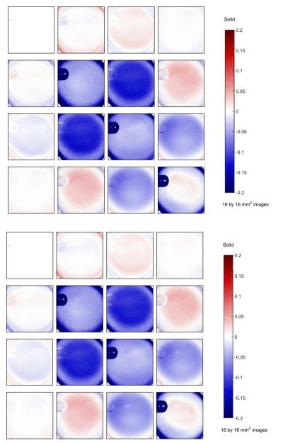
Figure 4.4: Logarithmically decomposed matrices  $L_u$  for the electro-optic BSO under exposure of the AC-driven plasma jet, shown before and after impact of the ionization waves, respectively in the top and bottom matrix. The diagonal elements represent the depolarization properties, while the off-diagonal elements are related to the uncertainties of the optical property elements of the  $L_m$  matrix.
