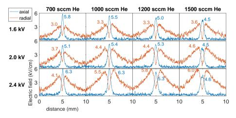
Figure 4.11: The vertical cross-section lines of the axial (blue) and radial (red) electric field going through the impact point for the electric field patterns obtained in dry air shown in figure 4.10. The maximum values of the radial and axial fields are denoted, with an estimated uncertainty of 0.3 kV/cm.
