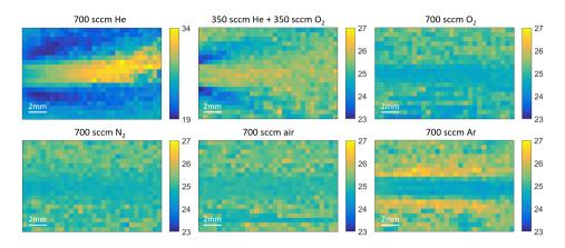
Figure 7.4: The mapped temperature profiles for different gas flows (helium, helium + oxygen, oxygen, nitrogen, dry air and argon) using the GaAs probe sensor. The ambient conditions are  $\approx 25$  °C. The end of the capillary is located on the left-hand side.
