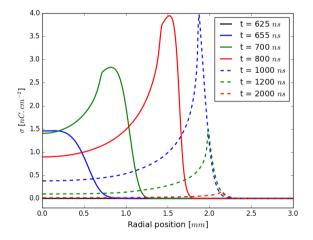
Figure 5.10: The surface charge density  $\sigma$  during the interaction of a guided ionization wave impacting on a glass target, as calculated by Pedro Viegas using an axysymmetrical numerical fluid model.
