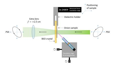
Figure 8.2: The adapted experimental setup (top view) shown of the Mueller polarimeter in between the *Polarizer State Generator* (PSG) and *Polarizer State Analyer* (PSA), including an additional lens and the translation stages to position both the sample (BSO crystal with onion cells) and the plasma jet. The other parts of the polarimeter remain the same as presented in chapter 2.
