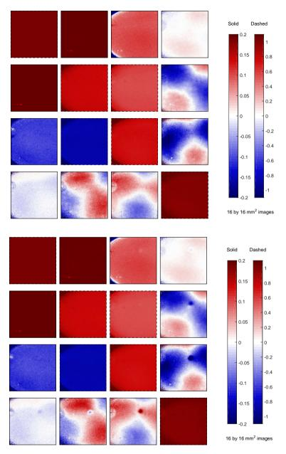
Figure 5.6: Mueller matrices obtained of the electro-optic BSO examined at 45 degrees under perpendicular exposure of guided ionization waves produced using a pulsed plasma jet operated using 4 kV pulses, measured time-resolved and shown before impact  $t_d = 0.2 \ \mu s$  (top) and after  $t_d = 0.7 \ \mu s$  (bottom). Hence, the second matrix includes the effect of temporally deposited surface charges. The image border (solid or dashed) indicates the colorscale.
