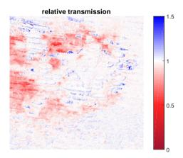
Figure 8.7: Transmission obtained from the two Mueller matrices measured timeresolved after impact (Mueller matrix 1,  $t_d = 7 \ \mu$ s) and before impact (Mueller matrix 2,  $t_d = 28 \ \mu$ s). The total accumulated time the sample has been under exposure is denoted by  $t_{exp}$  in minutes. The relative transmission between the time-resolved measurements is simply obtained by division between the transmission of the second matrix by the transmission of the first matrix.
