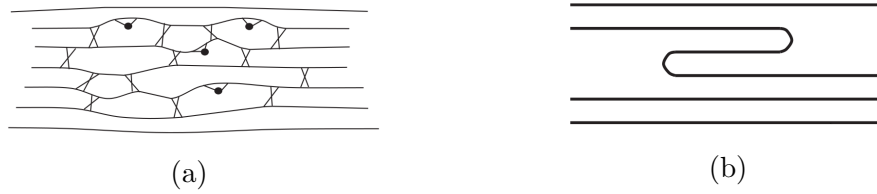
Figure 2.16: Schematic representation of a) the buckle and b) the ruck and tuck defects [HSMDH11].
