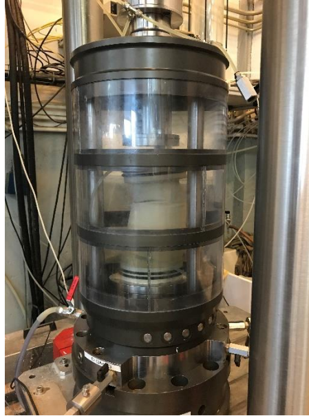
Figure 2.7 - Total collapse of a loose specimen of Fontainebleau sand
