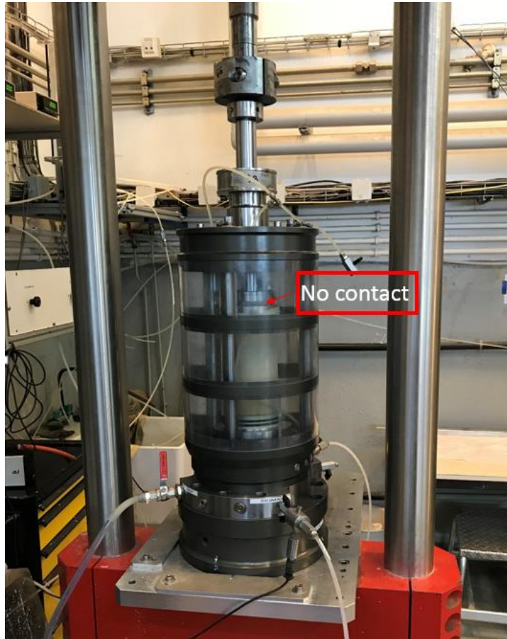
Figure 2.25 - Piston position during a monotonic test
