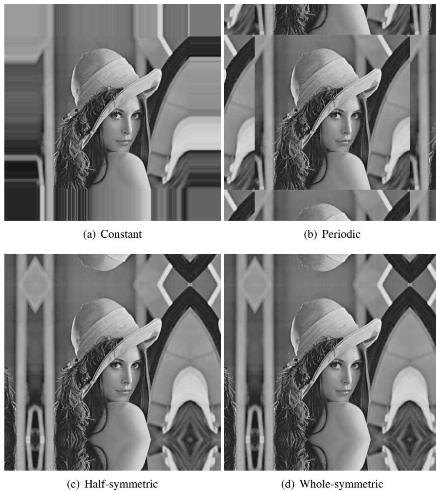
Figure 5.3: Extended image used during the prefiltering using Algorithm 5.3 for \epsilon = 10^{-8} i.e 8 digits and n = 11 . The image is extended of L_0^{(n,\epsilon')} = 125 pixels from its boundary.
