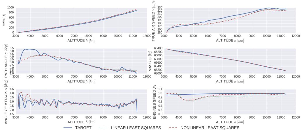
Figure 3.15 – Solution of problem (3.7.5) using dynamics estimated by single-task OLS (dotted green) and multi-task NLS (dashed red), in comparison to a recorded flight (full blue line).
