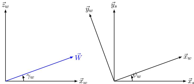
Figure 3.7 –  $\mathcal{R}_w$  rotation relative to  $\mathcal{R}_s$  ( $= \mathcal{R}_i$  in subsection 3.2.5).
