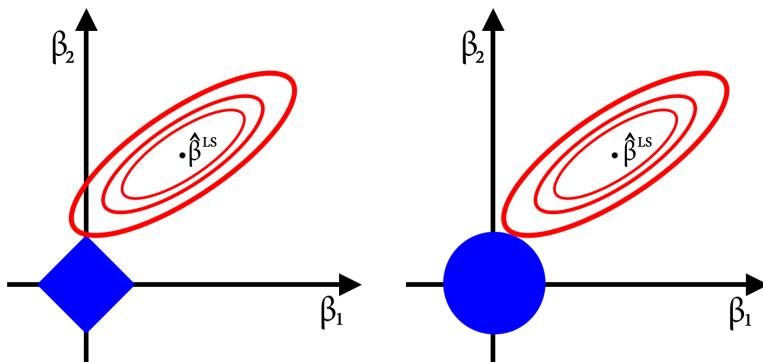
Figure 4.1 – The left frame shows the shape of the  $L^1$  constraint of the Lasso in blue, the contours of the least-squares criterion being represented by the ellipsoids. The right frame represents the same, but with the squared  $L^2$  constraint from the Ridge regression. The OLS solutions are denoted by  $\hat{\beta}^{LS}$  here.<sup>1</sup>
