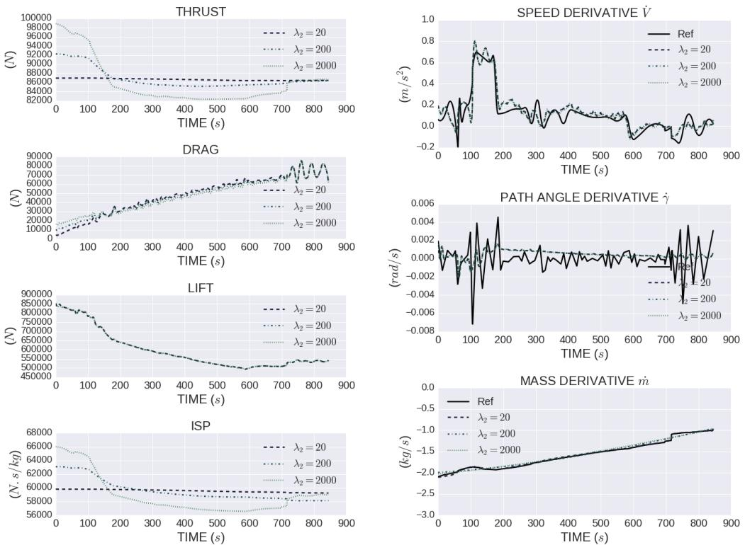
Figure 4.15 – (Left) Thrust, Drag, Lift and Specific impulse predicted for the test flight with different regularization parameters  $\lambda_2$ . (Right) Respective states derivatives predictions.
