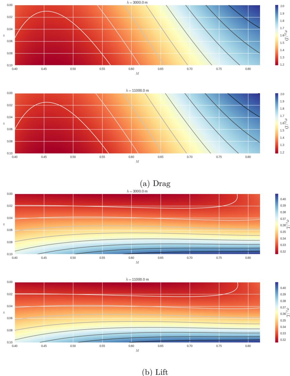
Figure 3.12 – Standardized dispersion (ratio of the standard deviation to the mean  $\sigma/\mu$ ) induced on the predicted drag  $\hat{D}$  and lift  $\hat{L}$  by the 50 local solutions found. As  $D$  and  $L$  depend on  $h, \alpha, M$ , each panel corresponds to a fixed altitude  $h$  and depicts the dispersion over a realistic range of  $(\alpha, M)$ .
