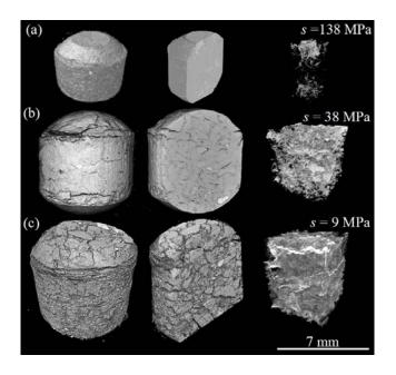
Fig. 3. X-ray computed microtomography ( $\mu$ -CT) observations (4.41  $\mu$ m/voxel) – 3D reconstruction image and network of cracks: (a) initial state; (b) s = 38 MPa; (c) s = 9 MPa; (d) s = 1 MPa.
