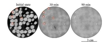
Figure 14. Evolution of the patterns of vertical sections of sample 2a upon wetting.
