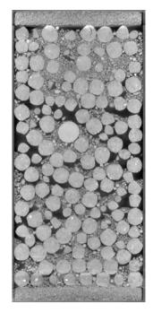
Figure 2. Vertical slice on the investigated pellet/powder bentonite mixture obtained by  $\mu$ -CT observations - Resolution: 50  $\mu$ m/voxel.
