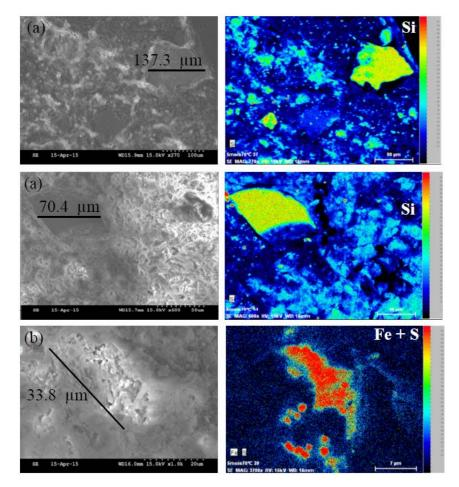
Figure 13. SEM pictures taken on a pellet of bentonite at its initial state (132.38 MPa of suction) + EDS results. Mineral inclusions of quartz (a, b) and pyrite (c). Dry unit mass  $\rho_d = 2.12 \text{ Mg/m}^3$ .
