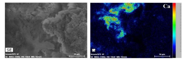
Figure 14. SEM picture taken on a pellet of bentonite at its initial state (132.38 MPa of suction) + EDS results. Mineral inclusion of calcite. Dry unit mass  $\rho_d = 2.12 \text{ Mg/m}^3$ .
