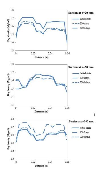
Fig. 26. Profiles of dry density for sample 1 at different positions after 200 days and 5000 days of hydration.
