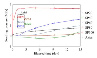
Figure 5. Evolution of the swelling pressure with time after 15 days of hydration.
