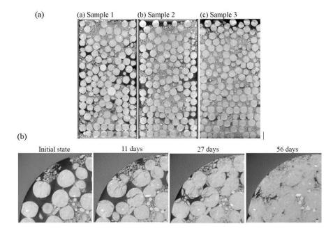
Fig. 9. (a)  $\mu$ -CT observations (vertical slices) of three different pellet/powder bentonite mixtures (image's resolution is 50  $\mu$ m/voxel). (b) Zoom at 60 mm from the bottom of the sample 1 at different times.
