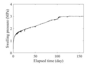
Figure 6. Evolution of the axial swelling pressure of the mixture.
