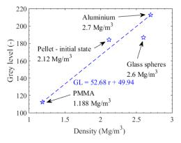
Fig. 19. Correlation plot between density and grey level obtained from the µ-CT observations.
