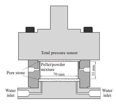
Figure 6. Constant-volume cell for swelling pressure determination.
