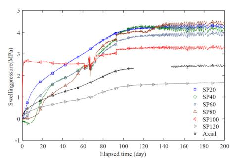
Figure 6. Evolution of the swelling pressure with time after 200 days of hydration.
