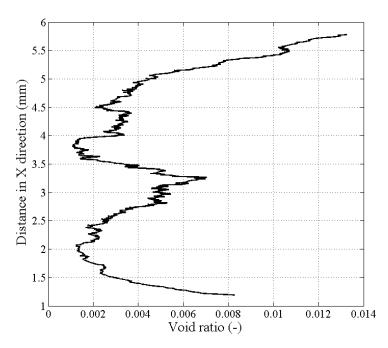
Figure 9. Evolution of the void ratio of a pellet of bentonite at initial state (X direction – vertical sections).
