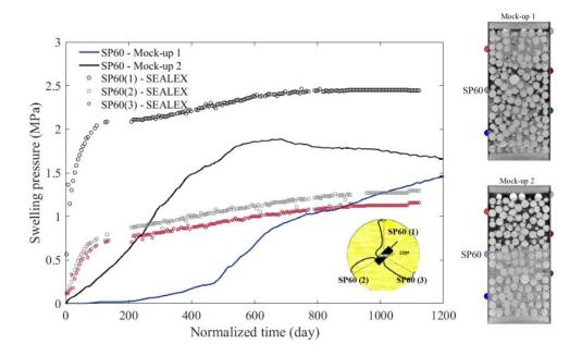
Figure 19. Comparison of swelling pressure results at 60 mm from the bottom hydration front for SEALEX *in situ* test and mock-up 1 test.
