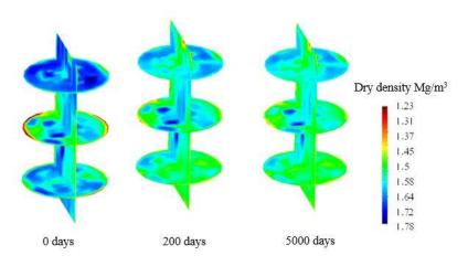
Fig. 27. Contours of dry density at different hydration times.
