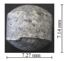
Figure 2. Pellet at initial state.
