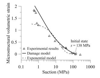
Fig. 14. Microstructural volumetric strain evolution upon wetting under free swelling conditions of MX80 bentonite pellets. Experimental data and the proposed damage model.
