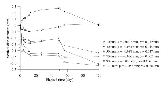
Figure 12. Vertical displacements obtained by Digital Image Correlation Technique (DIC) based on the PMMA spheres network while wetting.
