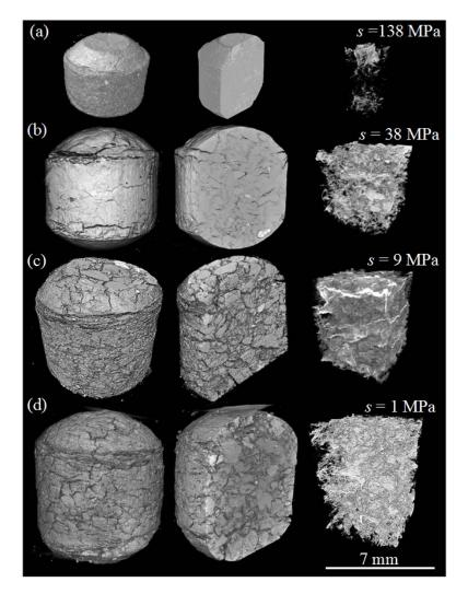
Figure 14. X-ray computed microtomography ( $\mu$ -CT) observations – 3D reconstruction image and network of cracks: (a) P0 – initial state ; (b) P4 – s = 38 MPa; (c) P6 – s = 9 MPa; (d) P8 – s = 1 MPa.
