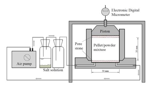
Figure 4. Experimental setup for suction-controlled oedometer tests.
