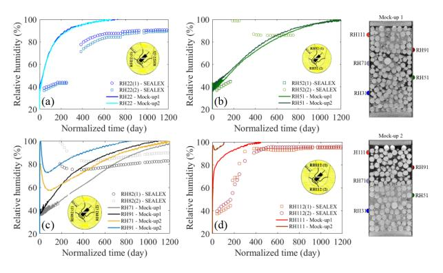
Figure 18. Comparison of relative humidity results between SEALEX *in situ* results and mock-up tests. (a) RH22; (b)RH52 for SEALEX test and RH51 for mock-up tests; (c) RH82 for mock-up tests, RH71 and RH91 for mock-up tests; (d) RH112 for SEALEX test, RH111 for mock-up tests.
