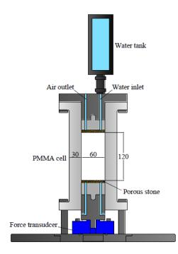
Figure 4. Layout of the transparent PMMA cell.
