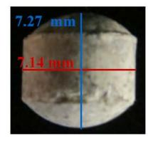
Figure 2. Pellet of bentonite at initial state. Dry unit mass  $\rho_d = 2.12 \text{ Mg/m}^3$ .
