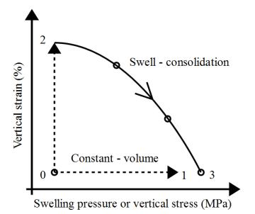
Figure 5. Swell-consolidation and constant-volume methods used to determine the swelling pressure.
