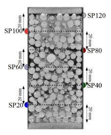
Figure 3. Vertical section of the investigated pellet/powder bentonite mixture obtained by  $\mu$ -CT observations. Resolution: 50  $\mu$ m/voxel.
