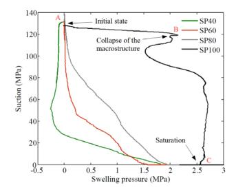
Figure 13. Suction versus swelling pressure at different positions.
