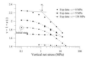
Fig. 17. Results from suction controlled oedometer tests on MX80 pellet/powder bentonite mixture (80/20) prepared at a dry density equal to 1.49 Mg/m<sup>3</sup>.
