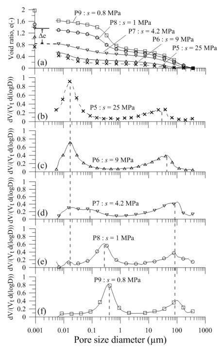
Figure 10. MIP tests results for P5-P9.
