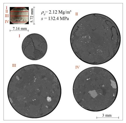
$\label{eq:Figure 4. X-ray computed microtomography (\mu-CT) observations - horizontal sections - of a \\pellet of bentonite at its initial state.$
