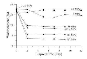
Figure 5. Water content versus elapsed time during path II for group B.
