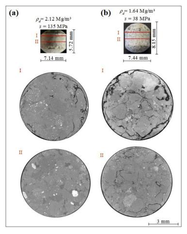
Figure 11. X-ray computed microtomography ( $\mu$ -CT) observations – horizontal section: (a) 135 MPa (P0); (b) 38 MPa (P4).
