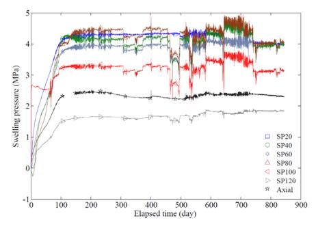
Figure 7. Evolution of the swelling pressure with time after 845 days of hydration.
