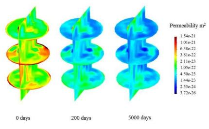
Fig. 28. Contours of permeability at different hydration times.
