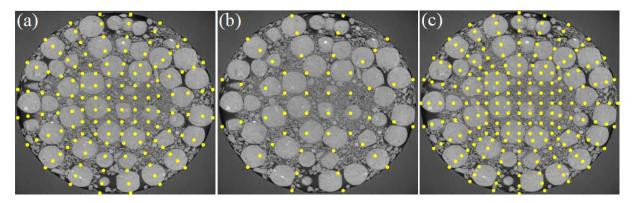
Fig. 29. Horizontal section of the sample 1 and finite element nodes corresponding to three finite element meshes used in the analysis.
