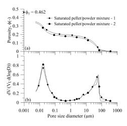
Fig. 7. MIP test results for two specimens of saturated pellet/powder mixture.
