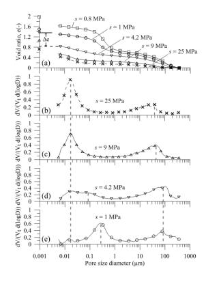
Fig. 5. MIP test results on a single pellet of bentonite equilibrated under suctions from 25
