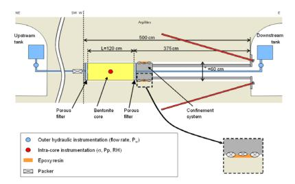
Figure 1. Layout of the SEALEX in situ tests (after Mokni et al., 2016).
