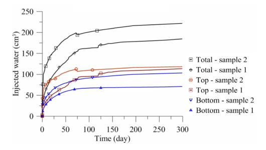
Figure 11. Volumes of injected water into sample 1 and sample 2 while hydration.
