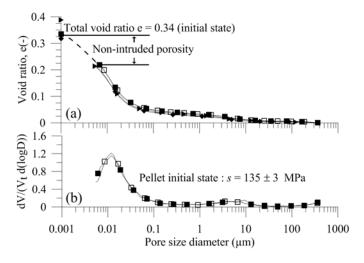
Figure 2. MIP tests results for a pellet of bentonite at its initial state.
