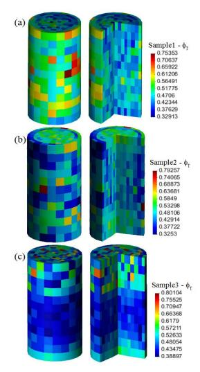
Fig. 20. Initial total porosity of the three samples.
