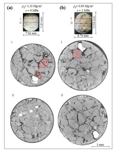
Figure 12. X-ray computed microtomography (μ-CT) observations – horizontal section: (a) 9 MPa (P6); (b) 1 MPa (P8).
