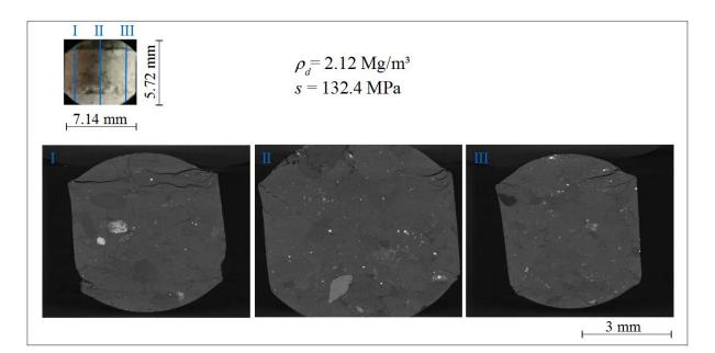
$\label{eq:Figure 5. X-ray computed microtomography (\mu-CT) observations - vertical sections - of a \\pellet of bentonite at initial state.$
