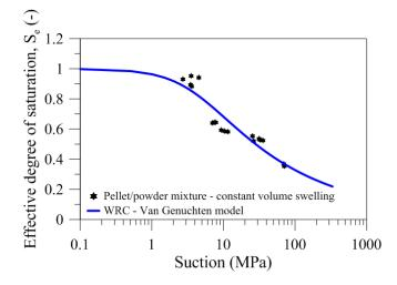
Fig. 16. Water retention curve of a MX80 bentonite pellet/powder mixture prepared at dry density of 1.49 Mg/m<sup>3</sup> under constant-volume conditions - experimental data and model fitting
