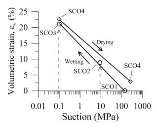
Figure 14. Volumetric strains measured at different suctions after equilibrium at the imposed suction for the different tests.
