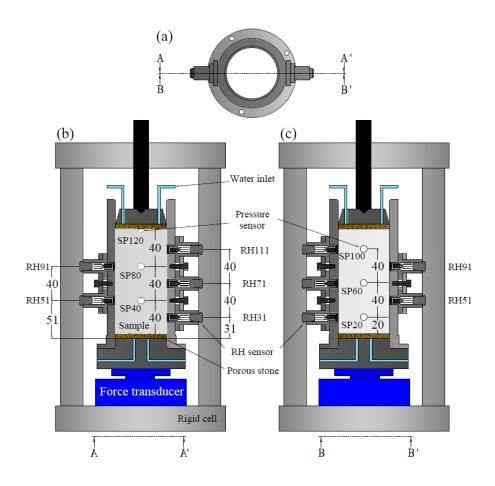
Figure 3. Layout of the mock-up test cell (a) top view; (b) section A-A'; (c) section B-B'.
