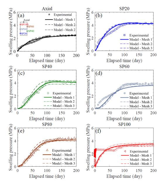
Fig. 30. Evolution of the swelling pressure at different positions with time -experimental data and model results with different mesh sizes.
