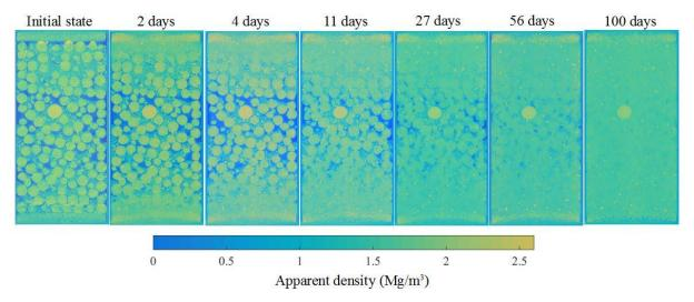
Figure 11. Apparent density field at various times.
