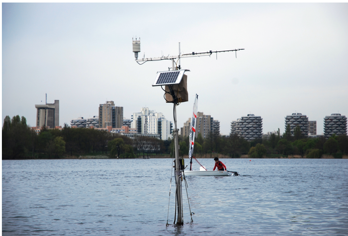
FIGURE B.1 : Station lac Precision Measurement Engineering, Inc. LakeESP installée au lac de Créteil (José Rodolfo scarati Martins)
