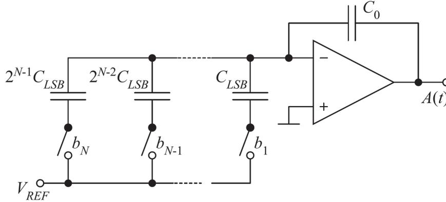
FIGURE 4.9: Illustration of an N-bit binary-encoded charge-redistribution DAC [11]
