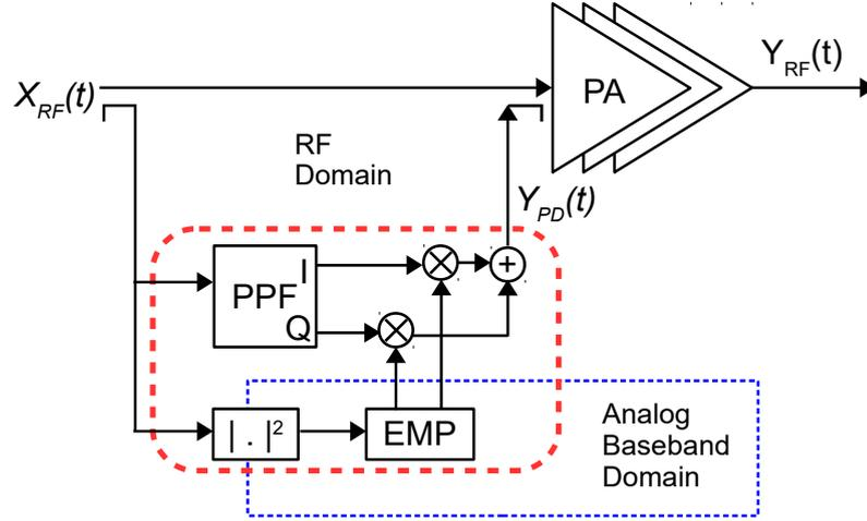
FIGURE 2.13: Block diagram of the ARFPD system of [8]
