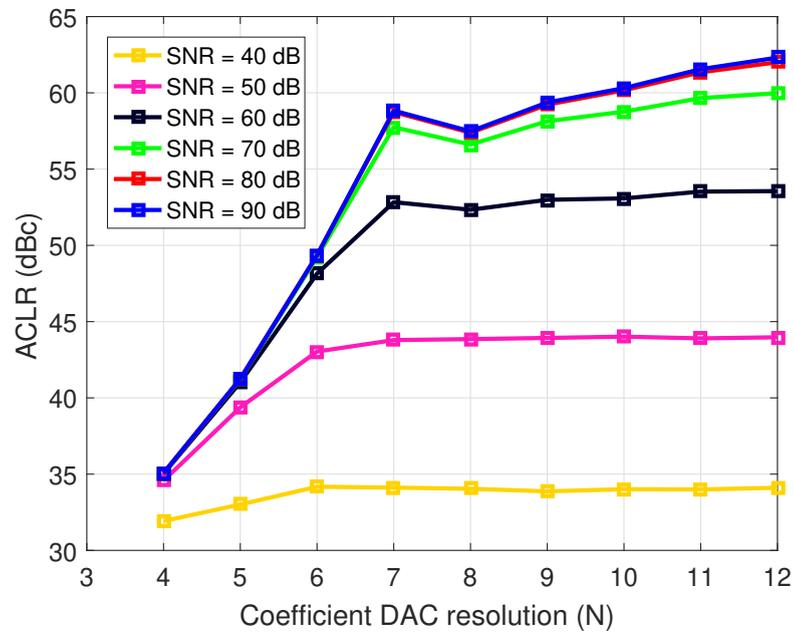
FIGURE 4.5: ACLR1 vs. coefficient DAC resolution, for various signal path SNR values, for the case of  $K = 9$  and  $M = 6$
