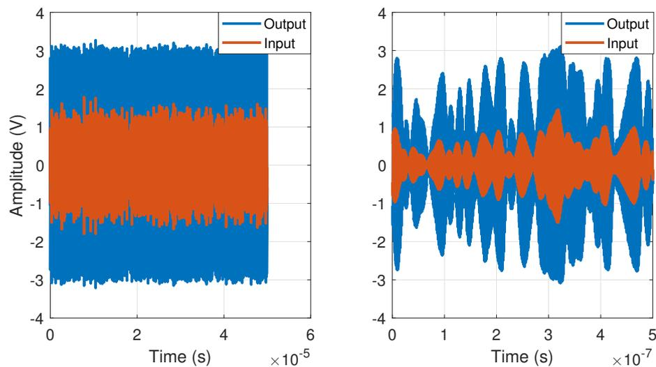
FIGURE 3.6: Measured PA input and output RF data from the oscilloscope sampled at 20 GSPS. Plots on the left is for the total captured duration, i.e.,  $50 \mu\text{s}$  and on the right is the time-magnified data for 50 ns duration
