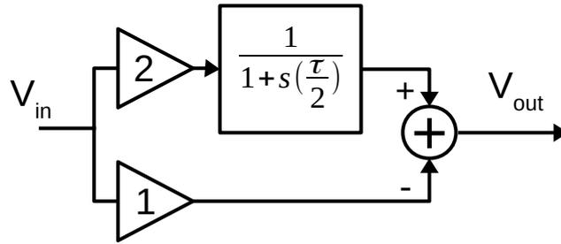
FIGURE 4.12: The block view of the first-order all-pass filter
