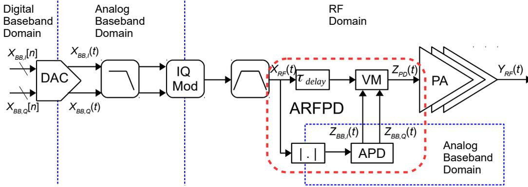
FIGURE 2.10: Block diagram of transmitter with ARFPD system
