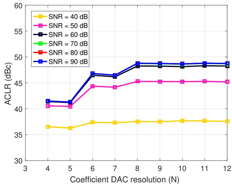
FIGURE 4.6: ACLR1 vs. coefficient DAC resolution, for various signal path SNR values, for the case of  $K = 5$  and  $M = 2$
