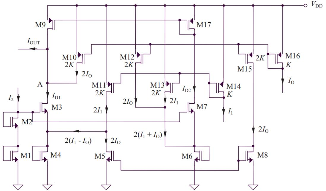
FIGURE 4.10: Current-mode multiplier circuit of [12]
