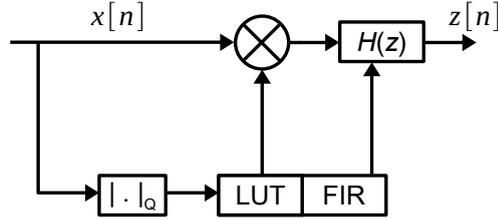
FIGURE 2.7: Block diagram of FLUT DPD of [4]
