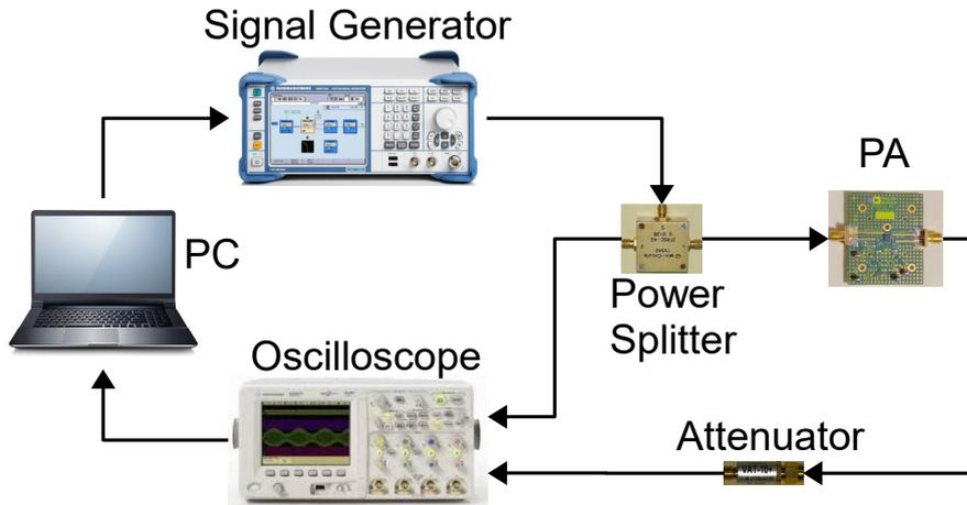
FIGURE 3.5: Measurement setup used for PA characterization
