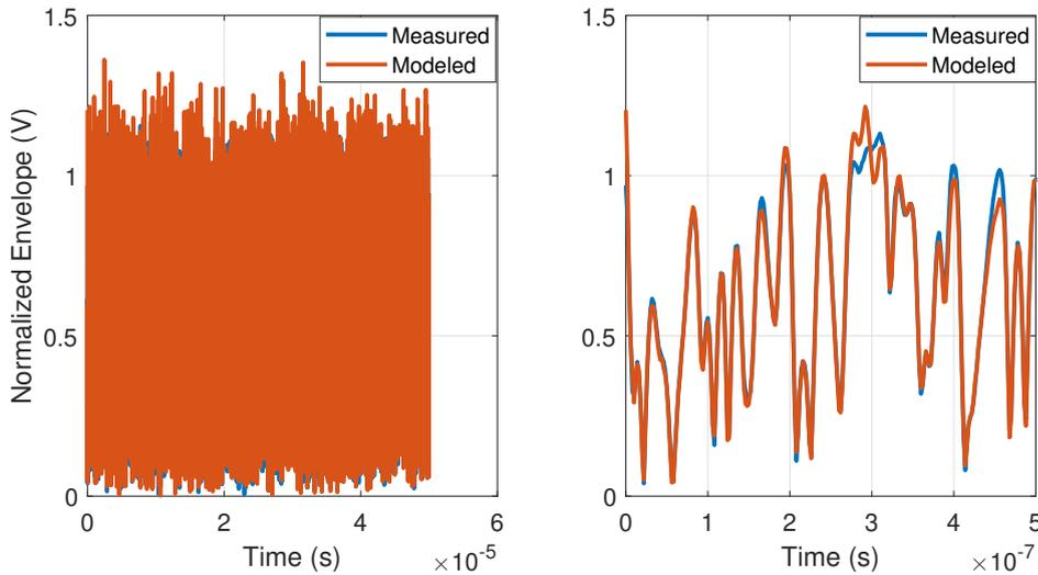
FIGURE 3.14: Plots of the measured and modeled PA output envelope. Plots on the left is for the total signal measurement duration of  $50 \mu\text{s}$  and on the right is the time-magnified data for  $50 \text{ ns}$  duration
