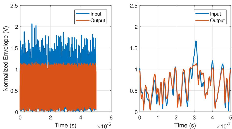
FIGURE 3.10: PA input and output baseband data envelope plots. Plots on the left is for the total captured duration, i.e.,  $50 \mu\text{s}$  and on the right is the time-magnified data for  $50 \text{ ns}$  duration
