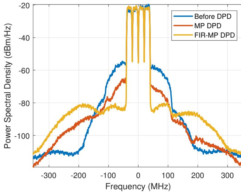
FIGURE 3.24: Power spectra of the output before and after linearization for a 4 carrier modulated signal with a total bandwidth of 80 MHz and PAPR of 8.5 dB. ACLR1 improvement of 15.6 dB is obtained using FIR-MP.
