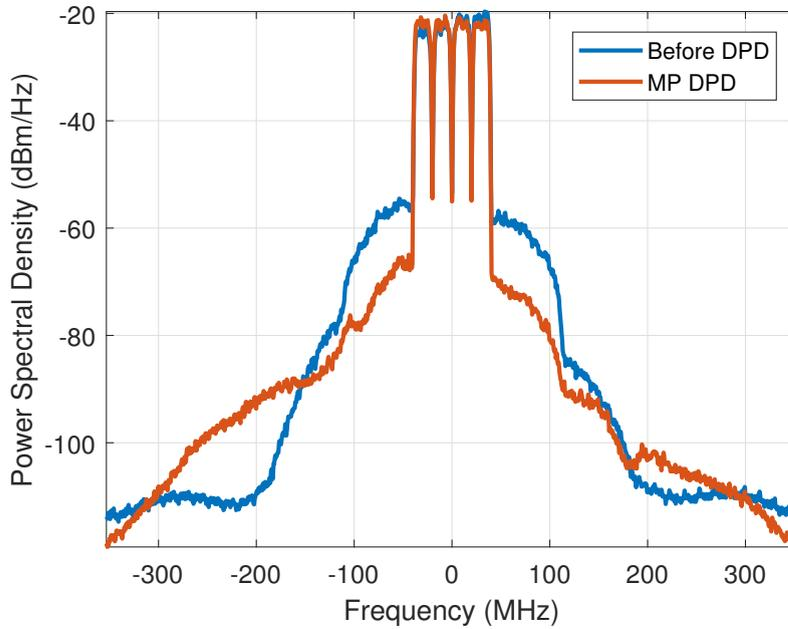
FIGURE 3.3: Power spectra of the output without and with MP predistorter for a 4 carrier modulated signal with a total bandwidth of 80 MHz and PAPR of 8.4 dB
