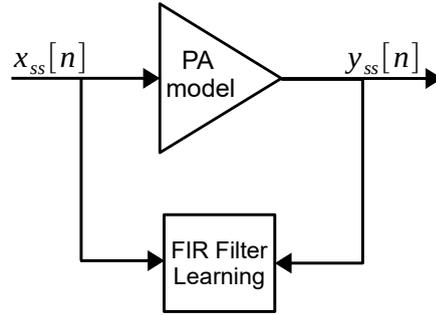
FIGURE 3.18: Illustration of FIR filter coefficients learning
