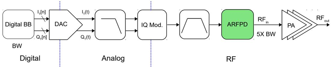
FIGURE 2.9: Illustration of a BS transmitter employing ARFPD system
