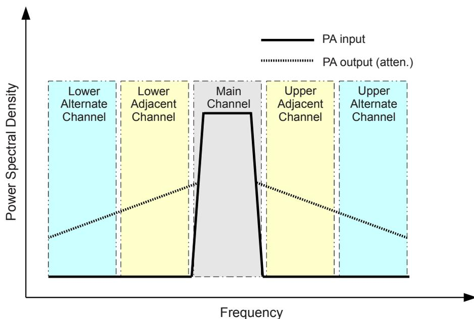
FIGURE 1.5: Illustration of PA input and output spectra
