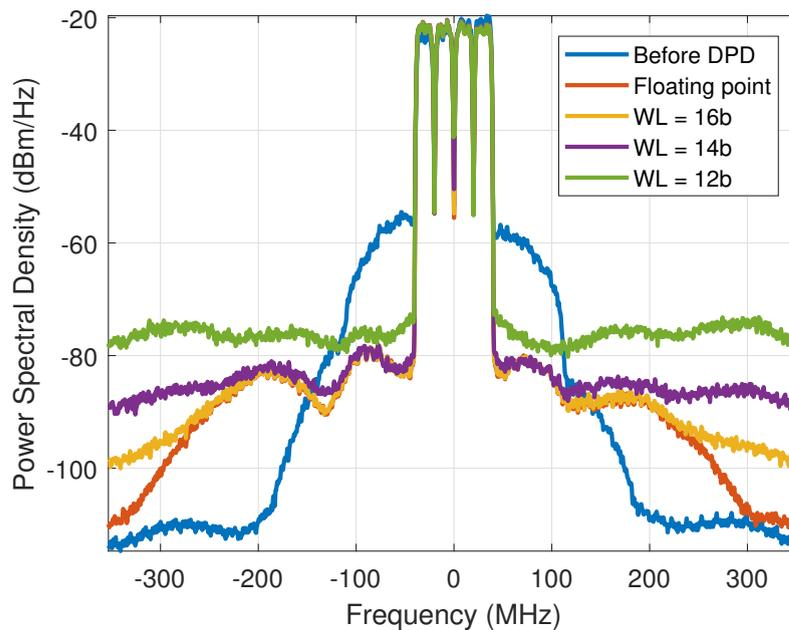
FIGURE 3.27: Spectra of the output signal without DPD and with floating-point and fixed-point representations of 16 bits, 14 bits and 12 bits for 80 MHz signal
