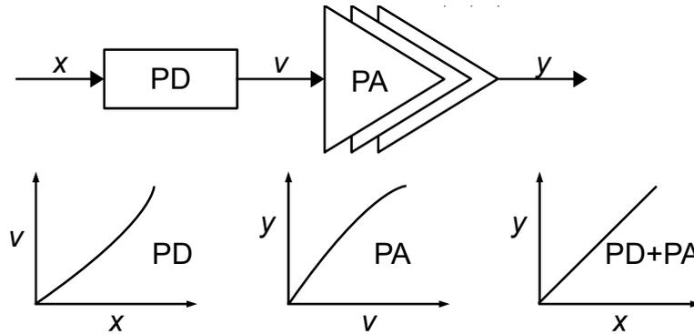
FIGURE 2.1: Illustration of the principle of PA predistortion
