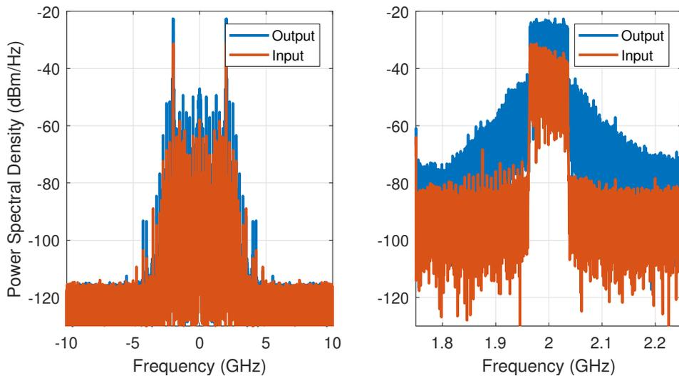
FIGURE 3.7: Spectra of the measured PA input and output RF data captured from the oscilloscope. Spectra on the left is for the total captured frequency, i.e., from  $-10$  GHz to  $10$  GHz and on the right is the frequency-magnified data from  $1.75$  GHz to  $2.25$  GHz
