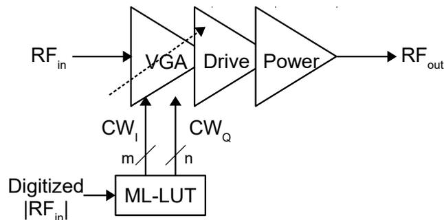
FIGURE 2.12: RFPD based PA driver stage of [7]
