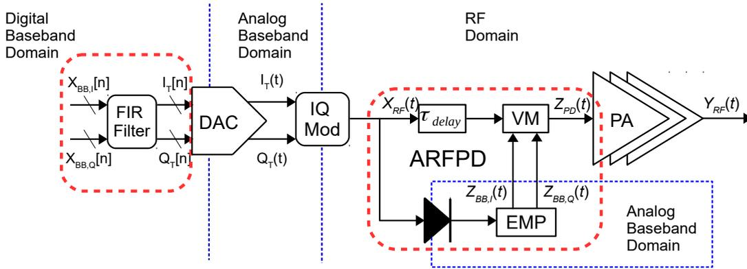
FIGURE 2.14: Block diagram of the FIR-EMP **ARFPD** [9, 10]
