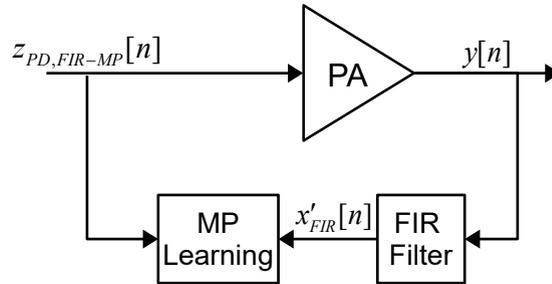
FIGURE 3.19: Illustration of MP block coefficients learning
