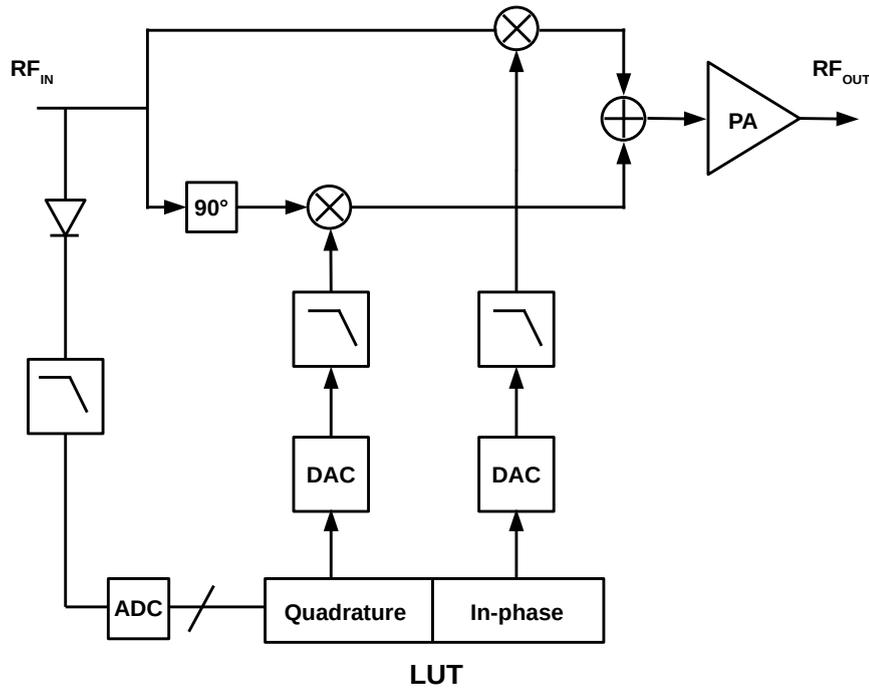
FIGURE 2.11: LUT based RF predistorter of [5, 6]
