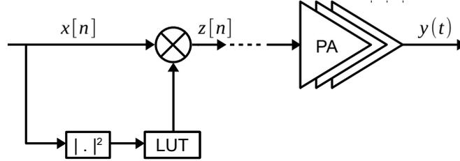
FIGURE 2.3: Gain based **LUT DPD** of [2]
