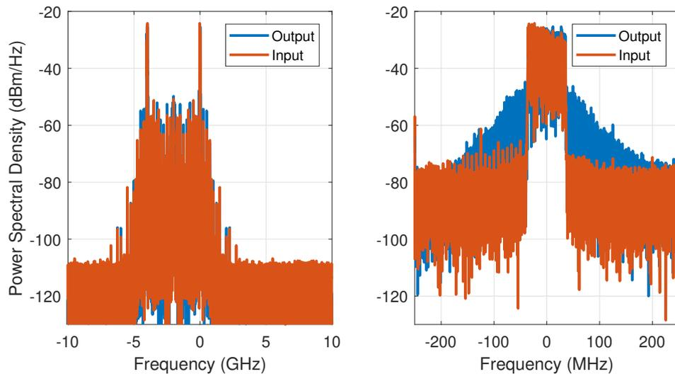
FIGURE 3.8: Spectra of the measured PA input and output downconverted and power-aligned data. Spectra on the left is for the total captured frequency, i.e., from  $-10$  GHz to  $10$  GHz and on the right is the frequency-magnified data from  $-250$  MHz to  $250$  MHz
