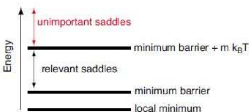
Figure 5.4 – Reaction mechanisms with barriers within mk_B T of the lowest saddle point energy are considered relevant (Xu & Henkelman, 2008).
