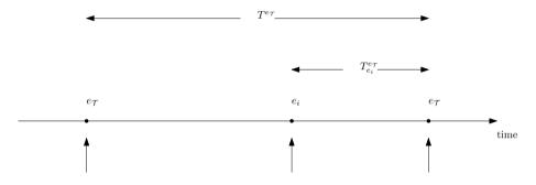
Figure 3.1: Survival time: Time interval between consecutive occurrence of a target failure  $e_T$  that occurs at times  $t_1$ and  $t_3$ .
