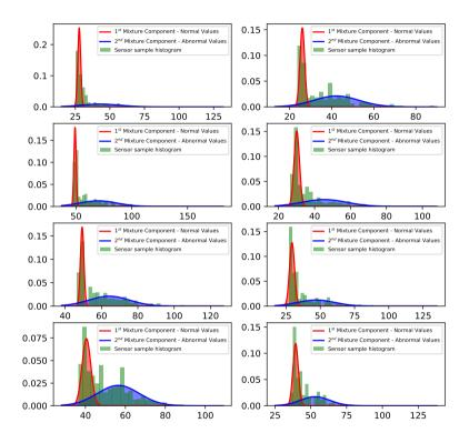
Figure 6.3: GMM fitted on 8 different sensors.
