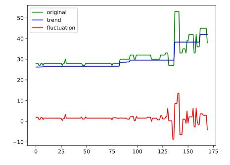
Figure 6.4: Decomposing the time series into the fluctuation and the trend
