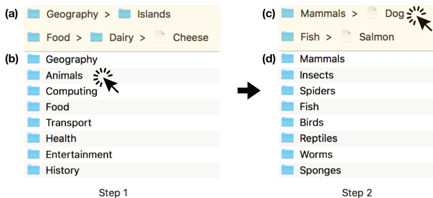
Figure 53: The BIGFile interface as the user navigates to “Dog” in a file retrieval task. (a) and (c) show the adaptive part with two shortcuts, (b) and (d) the static part. In Step 1, the shortcuts do not help and the user selects “Animals” in the static part, leading to Step 2 where the user directly selects “Dog” in the first shortcut, saving one navigation step.
