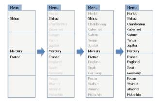
Figure 48: Ephemeral adaptation applied to menus: predicted items appear immediately, while remaining items gradually fade in. Taken from [58].
