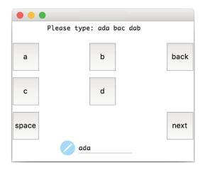
Figure 78: A toy keyboard with 7 keys: *a, b, c, d, space* (corresponding to character " " ), *back* represents backspace to erase the incorrect characters, *next* goes to the next sentence. The intended input X is shown above the keys and the currently transcribed sentence Y is indicated at the bottom.
