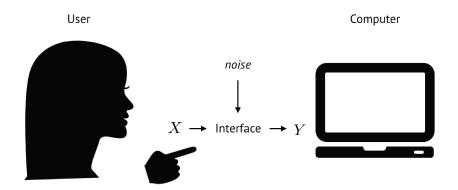
Figure 65: Information-theoretic measures for examining human-computer interaction as information transmission from the user to the computer through the channel interface. X is the intended input from the user and Y is the actual input received by the computer.
