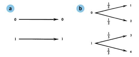
Figure 3: (a) Noiseless binary channel and (b) Noisy channel with nonoverlapping outputs (adapted from [34]).
