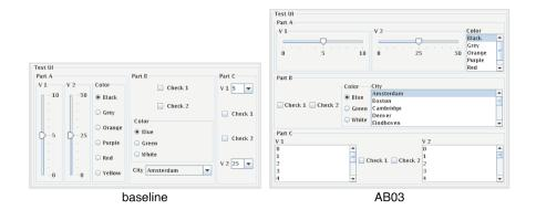
Figure 49: The baseline interface is shown in comparison to interfaces generated automatically by *SUPPLE* based on two participants' preferences. Participant ABo3 preferred lists to combo boxes but preferred them to be short. Taken from [73].
