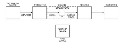
Figure 7: Schematic diagram of human motor system experiments as a model of communication system. Taken from [187].
