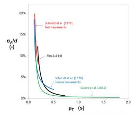
Figure 13: Guiard and Rioul's WHo model describing speed-accuracy tradeoff of aimed movement.  $\mu_T$  represents the average movement time;  $\sigma_A$  represents the standard deviation of movement amplitude; and d represents the distance to target center. Taken from [89].
