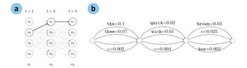
Figure 20: (a) Trellis of an observation sequence  $O = \{o_1, o_2, o_3\}$ . The thick arrows indicate an example of a highest probability path. (b) An example of a word confusion network [147].  $\epsilon$  represents a  $\epsilon$ -transition state to each observation index that allows a token to propagate to the next observation index without generating a corresponding letter. Figure taken from [165].
