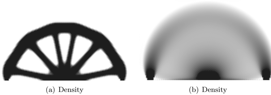
Figure 4.9: Optimized design of the bridge with penalized (a) and non penalized (b) SIMP method
