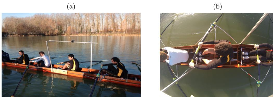
Figure 2.9: (a) Experimental set-up used to characterise the kinematics of the blade in water. A GoPro camera is installed above one of the rowers on the *eight* rowing boat from the *Ecole polytechnique* rowing club. The videos of the rower's hands are coupled with the measurement of the speed of the boat from a sensor based on GPS and accelerometer sensors. (b) Picture taken by the GoPro camera during the measurements.
