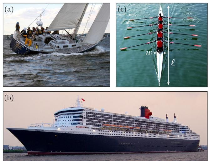
FIG. 1: Pictures of (a) a 44-footer sailing boat: length-to-width aspect ratio 3 and typical Froude number 0.6, (b) the *Queen Mary 2* liner: length-to-width aspect ratio 8.4 and typical Froude number 0.26, and (c) a coxless quadruple scull rowing boat: length to width aspect ratio 31 and typical Froude number 0.54. See Table I for details and characteristics of other boats.
