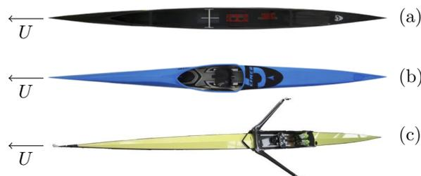
Figure 4.2: Pictures of (a) a sprint canoe, (b) a sprint kayak, and (c) a single scull rowing boat. The three boats are moving from right to left. Pictures have been rescaled (see Table 2.1 for the characteristics of rowing boats and Table 5.1 for the characteristics of sprint canoes and sprint kayaks).
