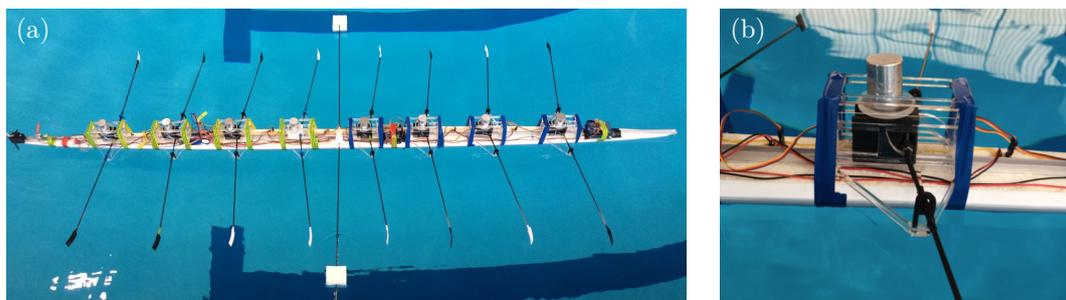
Figure 6.4: (a) Picture of our 2-meter long robotic rowing boat at the *Ecole polytechnique* swimming pool. (b) Zoom on one robotic rower. The blades are attached to a bar that can move up and down as the “rower” moves back and forth, thus mimicking the real rowing cycle.
