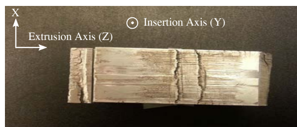
Figure 2.15: Specimen after 3 ECAP passes
