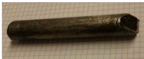
Figure 2.19: Batch B specimen after 6 ECAP passes following route Bc at 150°C.
