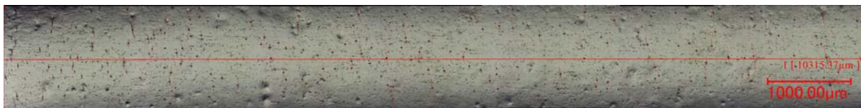
Figure 6.21: Counting and measurement of secondary crack along the gage-length of a UFG specimen subjected to a stress amplitude of 318 MPa.
