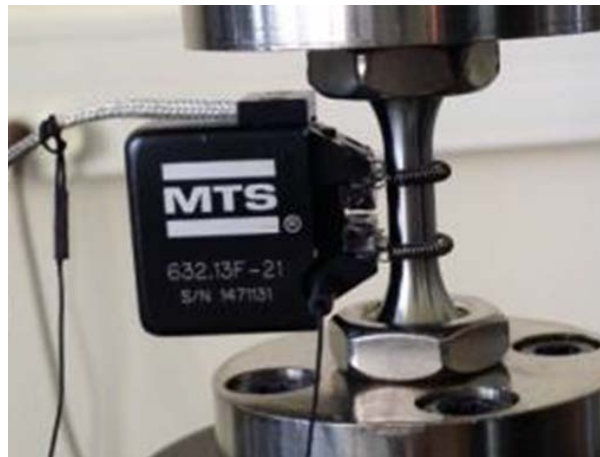
Figure 6.1: Mounted specimen with an extensometer for push-pull LCF tests.
