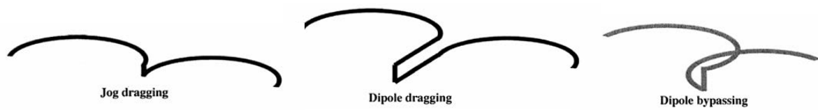
Figure 6.9: Schematics of dipole bypassing mechanism after jog dragging
