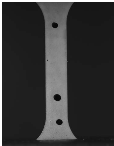
Figure 3.2: Macro-scale patterning for optical measurement of axial strain
