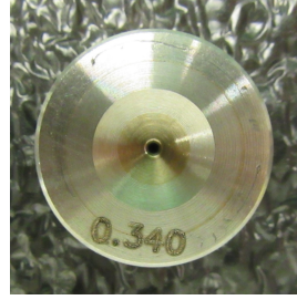
(b) Unused pinhole with aperture diameter marked on the piece.
