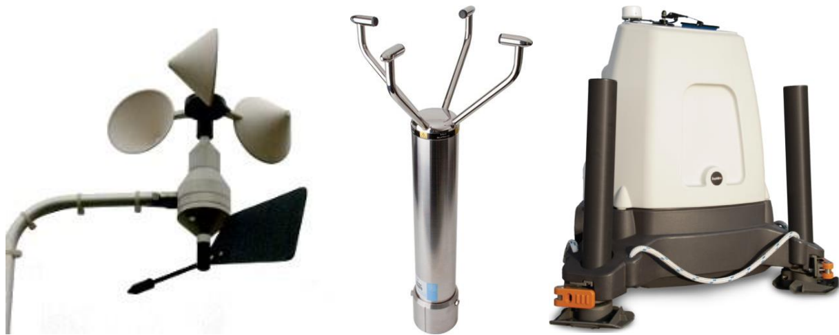
Fig. A3.1 Popular devices for wind velocity measurements: cup anemometer [117], ultrasonic anemometer [118], LIDAR [119]
