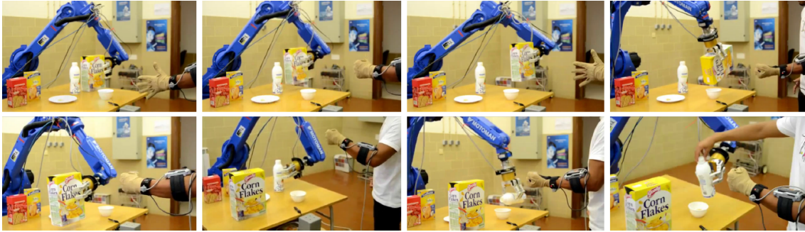
Figure 5.13: Visualization of different stages of robot teleoperation process: (a) starting point, (b) virtual joystick guidance to a goal, (c) forceful stop command, (d) rotation of the end-effector, (e) gesture-command to open the gripper, (f) grabbing a bottle and pulling it up, (g) rotation of the end-effector, (h) safe collaboration with the robot. NOTE: The virtual joystick mode moves the end-effector in a direction defined by the vector that joins a center position in which the hand is closed and the position of the hand when it is moved.
