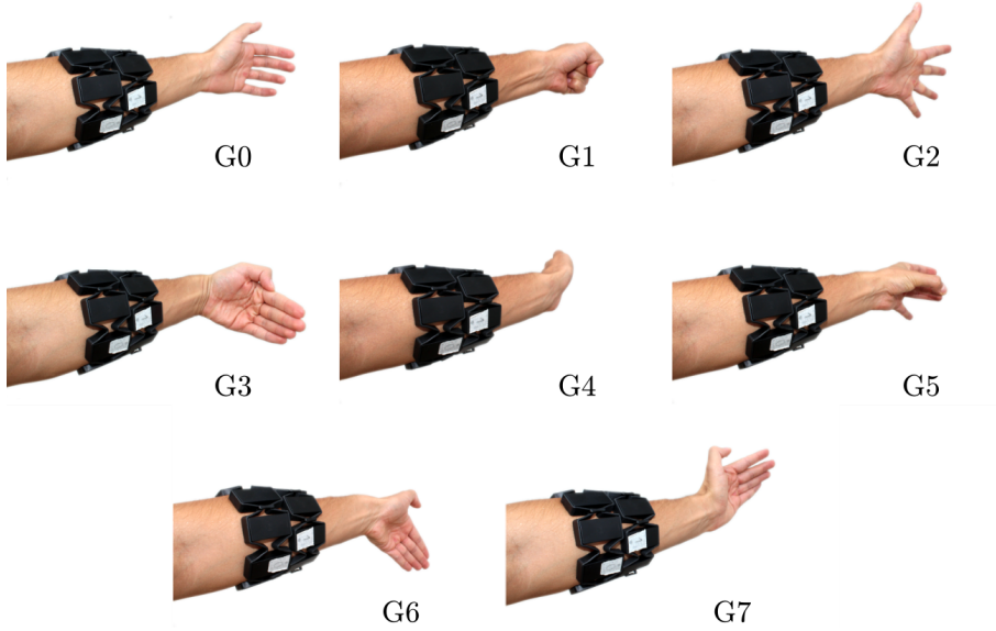
Figure 3.5: Representation of the library of gestures of the UC2018 DualMyo data set. By order, the gestures are: (0) rest, (1) closed fist, (2) open hand, (3) wave in, (4) wave out, (5) double-tap, (6) hand down, (7) hand up.
