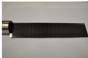
Fig. 2. Left: Rigid thin carbon flat plate of dimensions 3 mm (thickness) \times 191 mm (width) \times 40 mm (length). Right: PIV field of view at mid-span of the pitching plate inside the water-channel.
