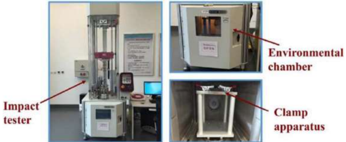
Figure 21: Experimental equipment used for low velocity impact tests. [227] Copyright
