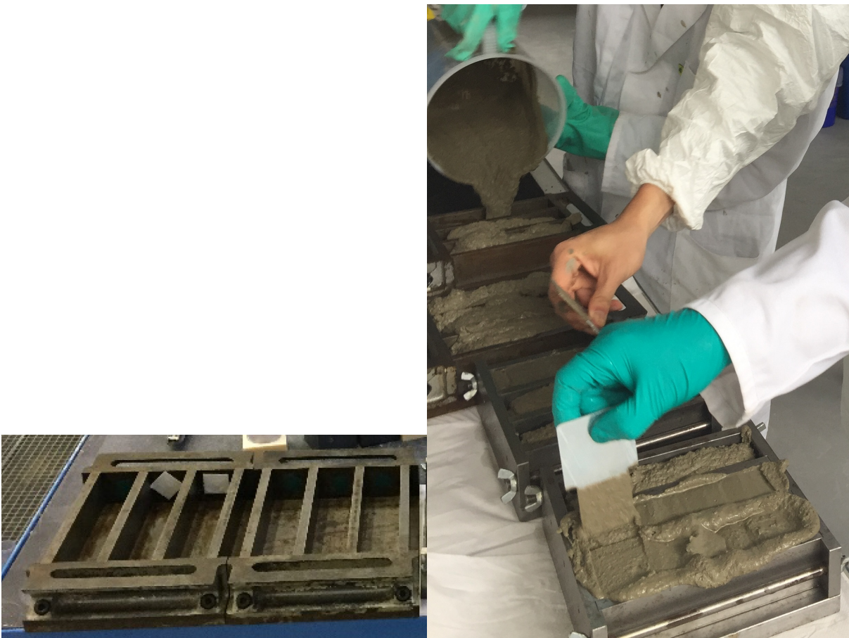
FIGURE 8.6 : Photos of the parallelepipedic metal molds ( 4cm \times 4cm \times 16cm ) (Left : empty molds ; Right : molds during the manufacture of specimens).
