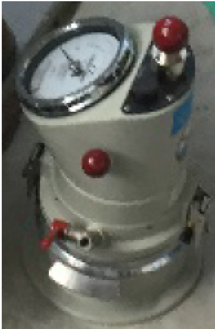
FIGURE 8.11 : Equipment to carry out the Aerometer test (1 liter).
