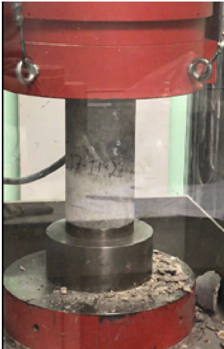
FIGURE 9.14 : Compressive strength test on the VeRCoRs concrete at CEA LECBA.
