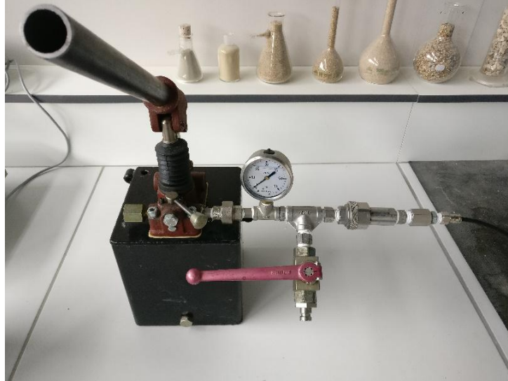
FIGURE 8.13 : Manual water pump.
