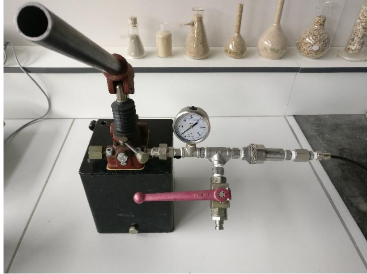
FIGURE 8.13 : Manual water pump.
