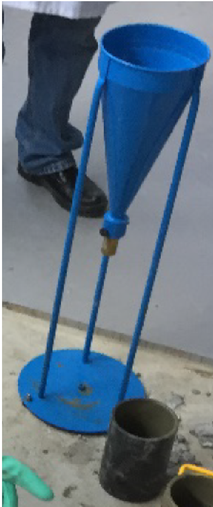
FIGURE 8.10 : Equipment to carry out the Marsh Cone Fluidity (EN445) Lab Test.
