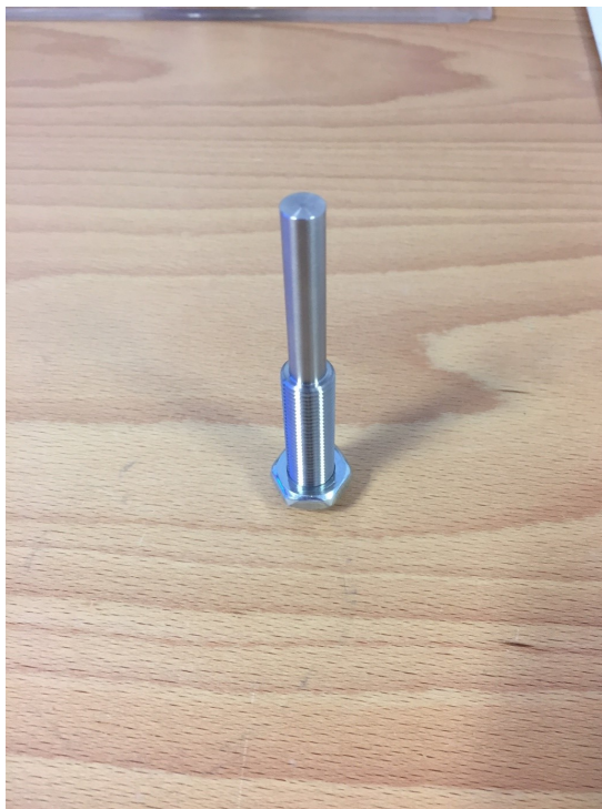
FIGURE 9.19 : Screw/nut system used to adjust the range of the displacement sensors.
