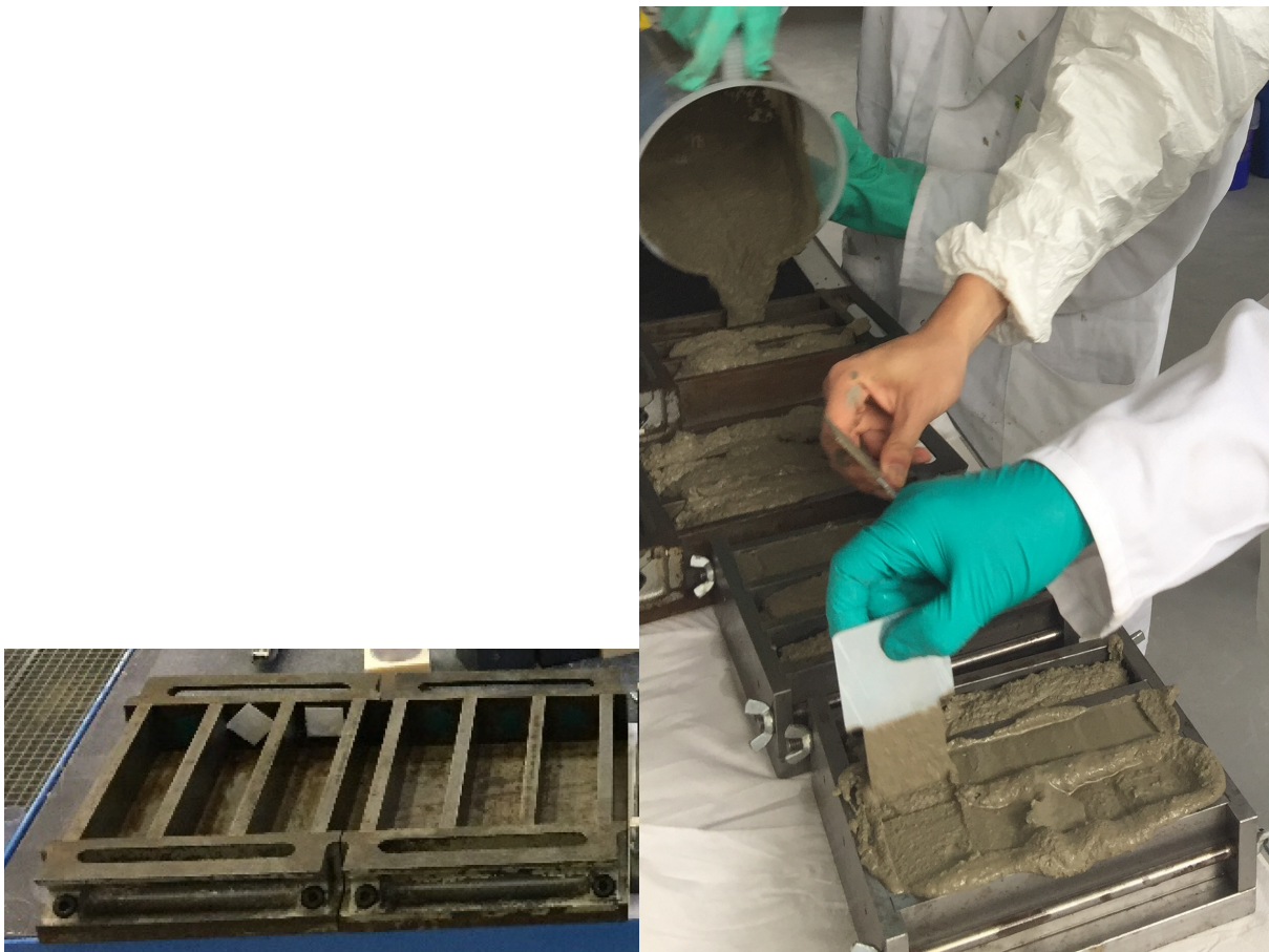
FIGURE 8.6 : Photos of the parallelepipedic metal molds ( 4\text{cm} \times 4\text{cm} \times 16\text{cm} ) (Left : empty molds ; Right : molds during the manufacture of specimens).
