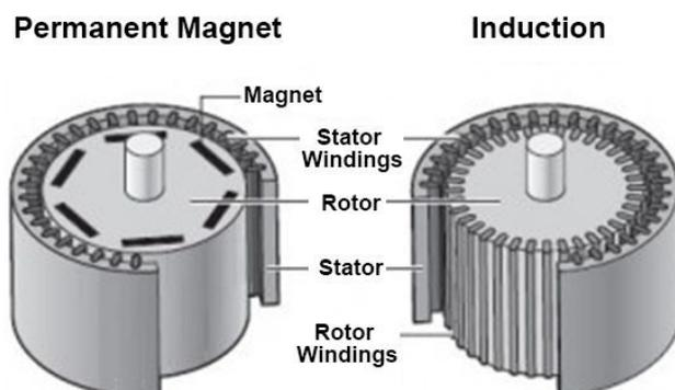
Figure 12.1: Permanent Magnet vs Induction Motor
