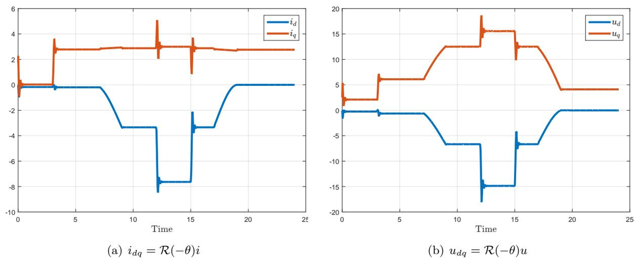
Figure 14.2: Currents and voltages in the rotating frame.
