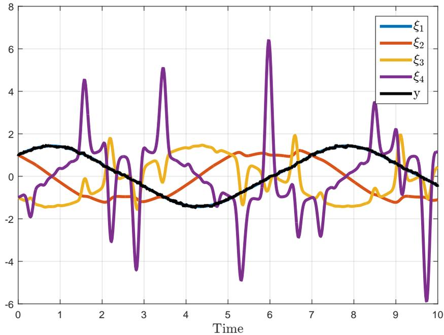
Figure 4.1: Trajectory of System (4.27), with initial condition  $\xi = (1, 1, -1, -1)$ , with input  $u = 5 \sin(10t)$  and with the noisy measurement  $y$  (filtered gaussian noise with standard deviation  $\sigma = 0.03$  and 1st order filtering parameter  $a = 50$ ), used to test the observers.
