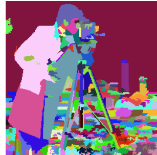
(f) Lambda-labelling of the output of the second watershed transform, using the labels image with small areas removed as marker image.
