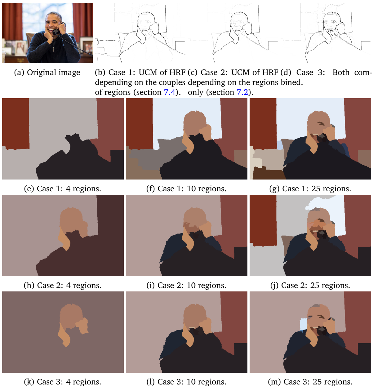
Figure 7.14 – Hierarchical segmentation of faces highlighting transitions between background and foreground.
