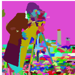
(h) Final labels image output by a watershed transform using previous labels image as marker.
