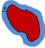
Figure A.6: Graphic representation of the proximity relation. The reference structure is depicted in red, the proximity region is depicted in blue.
