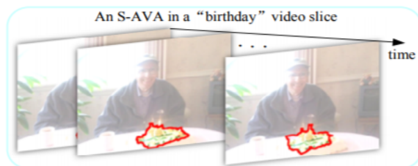
Figure 2.2. Example of an S-AVA taken from (Jiang et al., 2009a). The cake region track and the background birthday music form a salient multimodal atom for this event.
