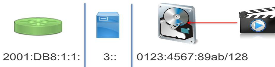
**Figure 2.1: Example of a routable object replica IPv6 address decomposition.**
